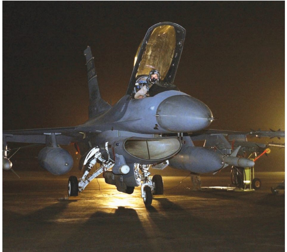
A South Carolina Air National Guard F-16C Fighting Falcon aircraft from the 157th Expeditionary Fighter Squadron, 379th Air Expeditionary Wing, is recovered following a nighttime mission at a forward deployed location during Operation Iraqi Freedom. The aircraft is armed with AIM-120B Advanced Medium Range Air-to-Air Missiles, AIM-9 Sidewinder missiles, and AGM-88 High-Speed Antiradiation Missiles, March 23, 2003. (Photographer: SMSgt Edward E. Snyder. Air Force Photo.)
