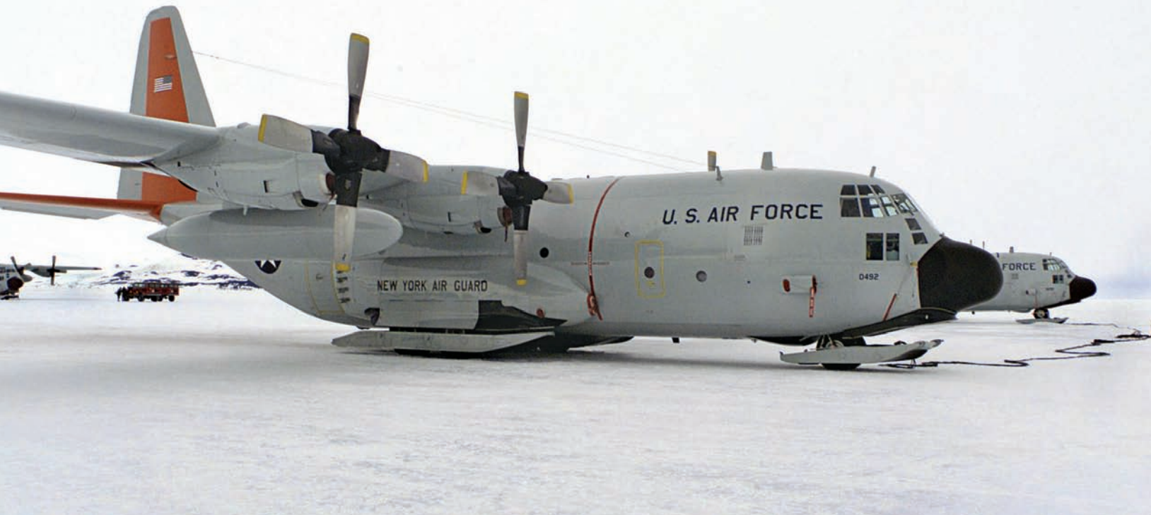
LC-130Hs equipped with landing skis, operated by the 109th Airlift Squadron, New York Air National Guard, parked on the ice pack at McMurdo Station at Ross Island in Antarctica during Operation Deep Freeze 2001. The unit operates six LC-130s between Christchurch, New Zealand, and a number of U.S. National Science Foundation stations located on the Antarctic ice pack, November 5, 2001. (Photographer: MSgt Joe Cupido. Air Force Photo.)
