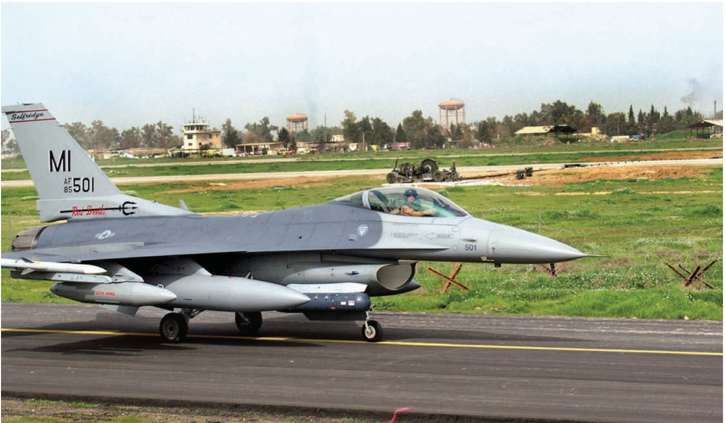
An F-16C Block 30, 107th Fighter Squadron, 127th Wing, Michigan ANG, carrying LITENING II pods in Kirkuk, Iraq. The 107th was the first F-16 unit in the Total Air Force to be based in Iraq. (Photographer: MSgt Glenn Wilkiwitz, Air National Guard. Air National Guard Photo.)
