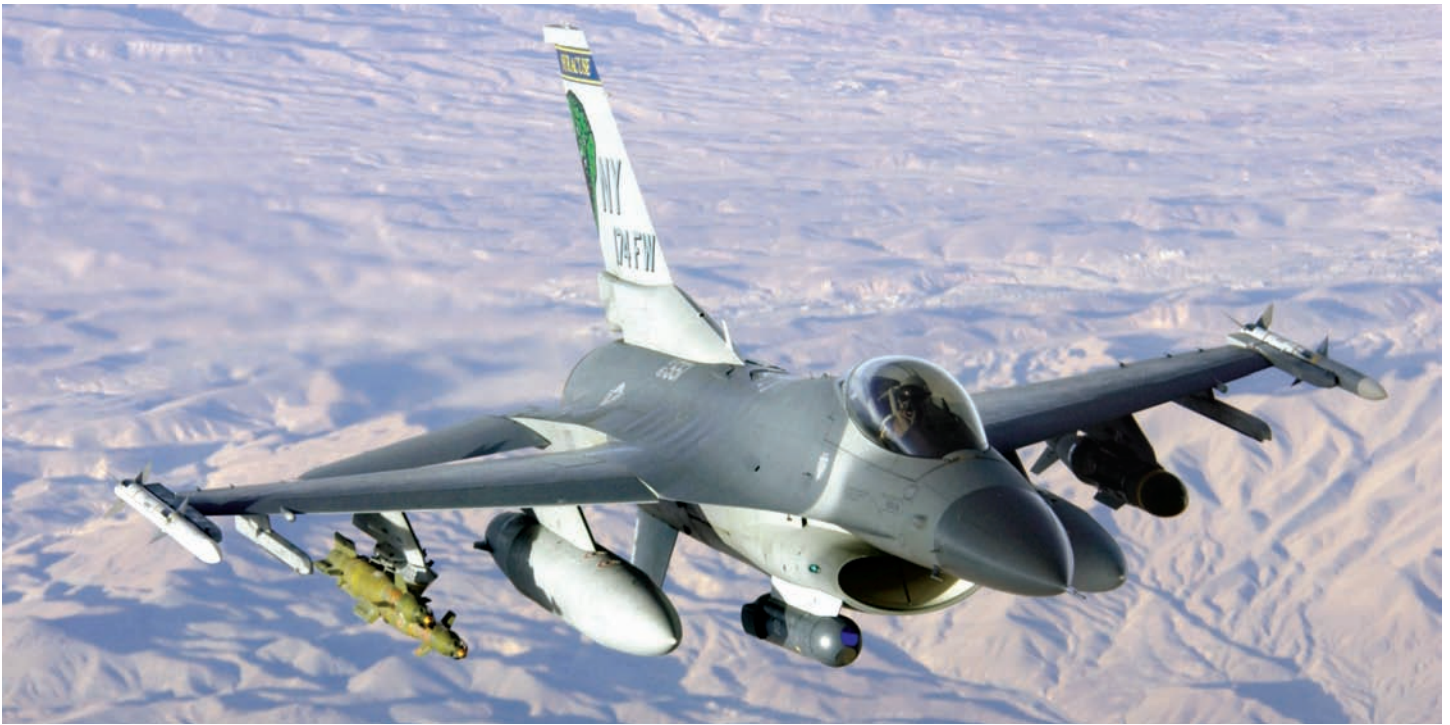
A US Air Force F-16C Fighting Falcon, 174th Fighter Wing, New York Air National Guard, Syracuse, New York, in flight over Afghanistan during Operation Enduring Freedom. The aircraft is armed with AIM-120A Advanced Medium Range Air-to-Air Missiles on each wing tip, a pair of GBU-12 500-pound bombs (left), a 370-gallon tank. It also has an AN/AAQ-28(V) LITENING II targeting pod under the intake, November 29, 2003. (Photographer: SSgt Suzanne M. Jenkins, USAF. Air Force Photo.)
