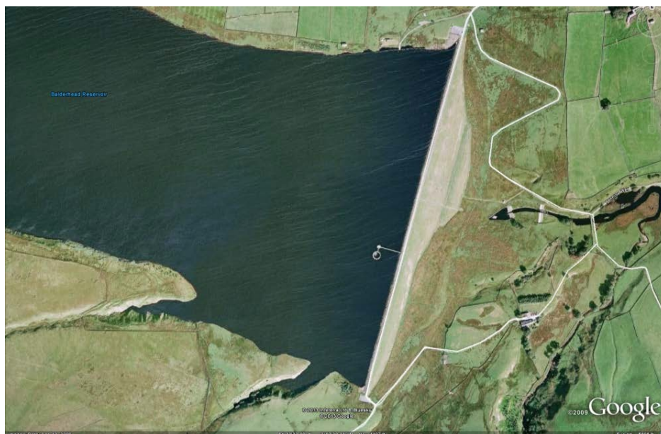
Figure 1.—Aerial view of 3,000-ft-long Balderhead Dam (Google Earth), which was the tallest earthfill dam in England when constructed.
