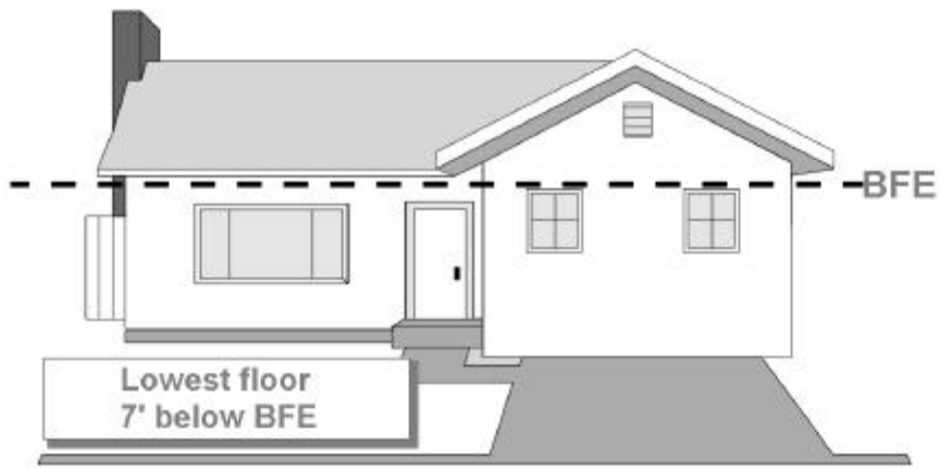
Figure 7-7. Pre-FIRM building—1995 insurance rate: $595
