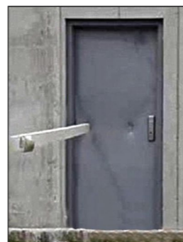
Tornado safe room impact test results: Door assembly passed; no perforation or latch/lock failure
