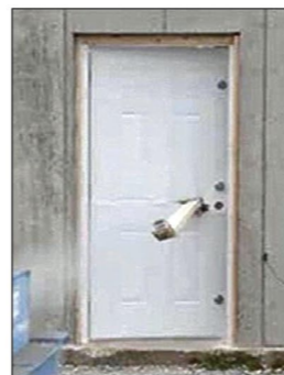
Tornado safe room impact test results: Door assembly failed when perforated
