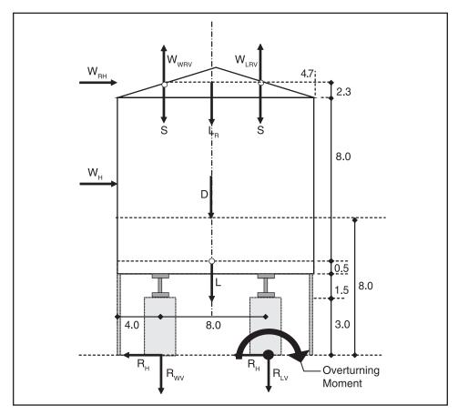
Figure F-3. Loading on a manufactured home.
