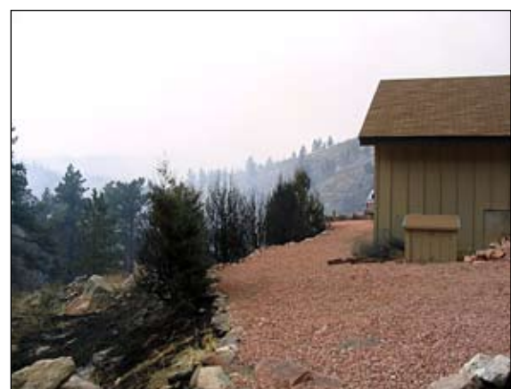
Figure 4. A noncombustible ground cover in Zone 1 helped this home survive a wildfire (Anchor Point Group, Boulder, CO).
