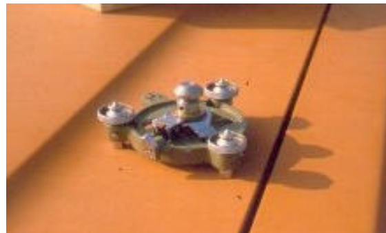
Figure 2-9. Target plug set on concrete structure. Forced centering device on tribrach shown upside down
