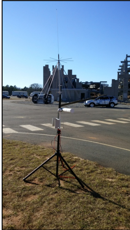
Figure 11. Diamond D3000N Broadband Super Discone Antenna Mounted to a Tripod Stand The specifications of the D3000N are:
