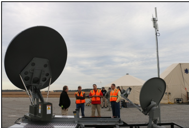
Figure 53. MED-1 Communications Antennas
