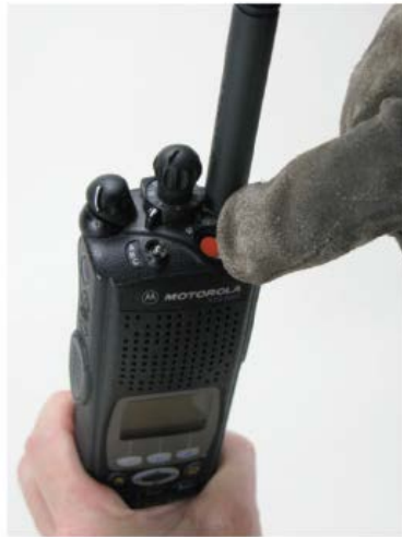
Figure 2. Inaccessibility of the Emergency Button Due to Small Size When Used With Thick Fire Gloves [23]
