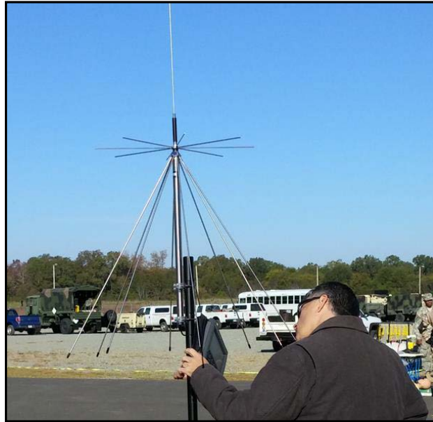
Figure 34. Keysight Fieldfox and Broadband Discone Antenna Used for Data Collection
