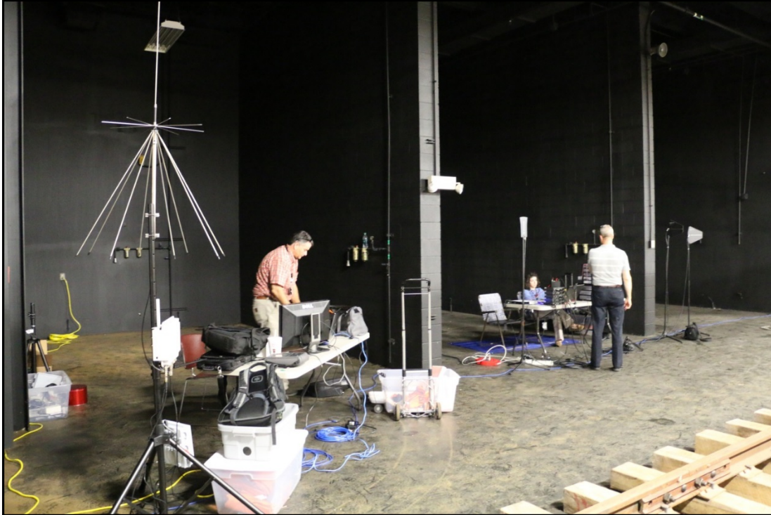
Figure 19. Radio frequency (left) and human factors (right) data monitoring stations for the subway exercise GPS time synchronization of the human factors data with the RF data was provided using an Ambient Clockit ACC501 time controller with a GPS receiver. The time was output by the Clockit as longitudinal time code (LTC), which is an audio-encoded time signal that can be synchronously mixed as a separate channel in the audio recording.
