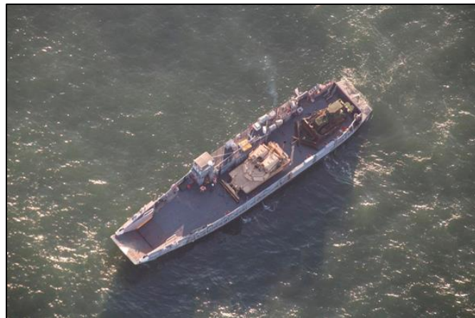
An ABV with combat dozer blade and an MCT with a mine rake embarked on an LCU.
