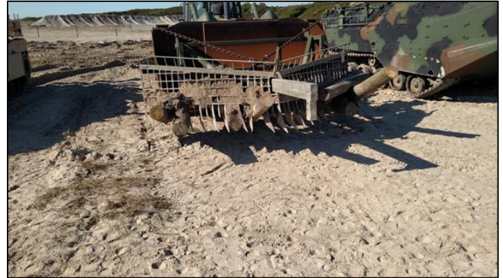
MCT mine rake after breaching operations with log obstacle remnants lodged in the teeth.
