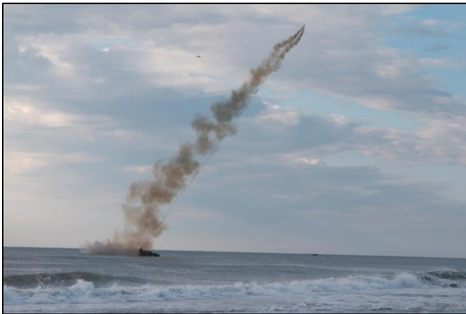
An Amphibious Assault Vehicle fires the Mk22 rocket and M58 line charge using the Mk154 launching mechanism.
