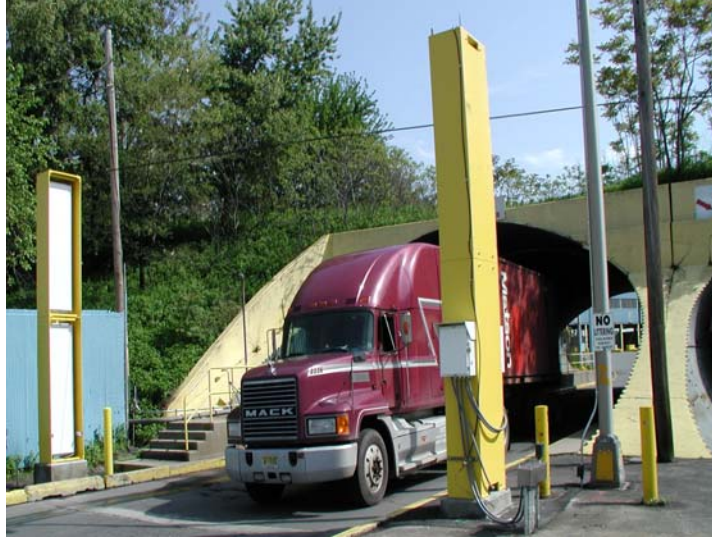
TEST-BED VENUE DEPLOYMENT OF RADIATION PORTAL MONITORS
