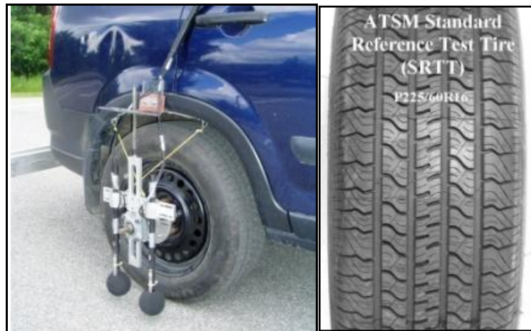
Figure 40. OBSI dual probe system and the SRTT.
