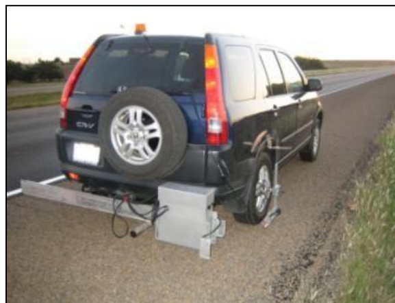
Figure 42. High-speed inertial profiler mounted behind the test vehicle.
