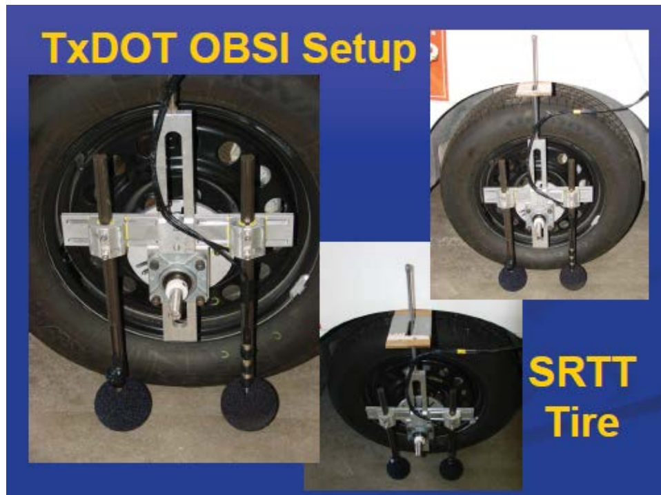
Figure 17. TxDOT OBSI Setup
