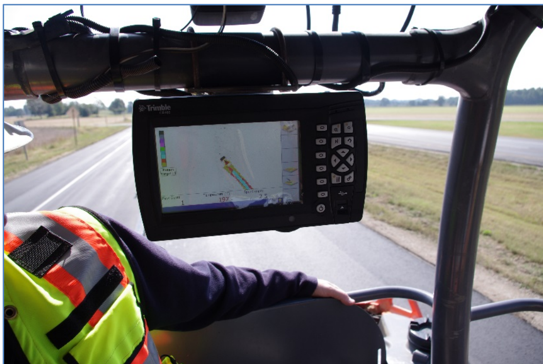
Figure 3. Photo. Roller-mounted computer screen used for real-time compaction information. (courtesy: University of Tennessee, Knoxville)
