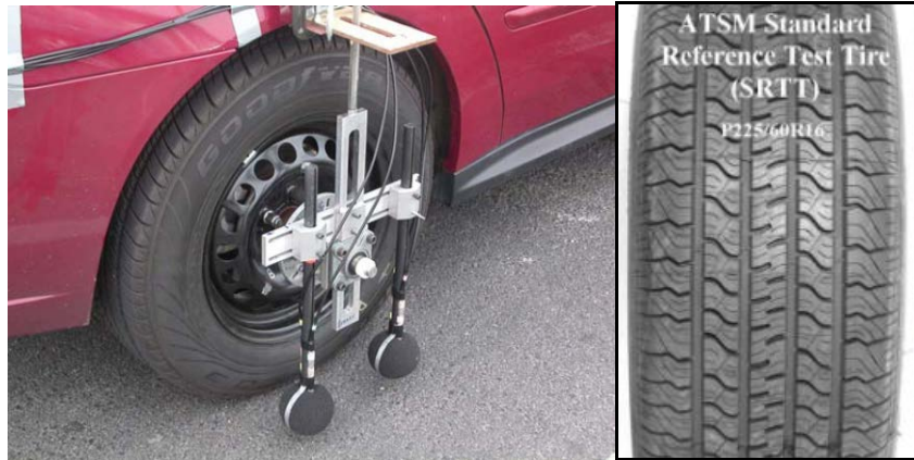
Figure 16. OBSI dual probe system and the SRTT. (Source: NCAT)
