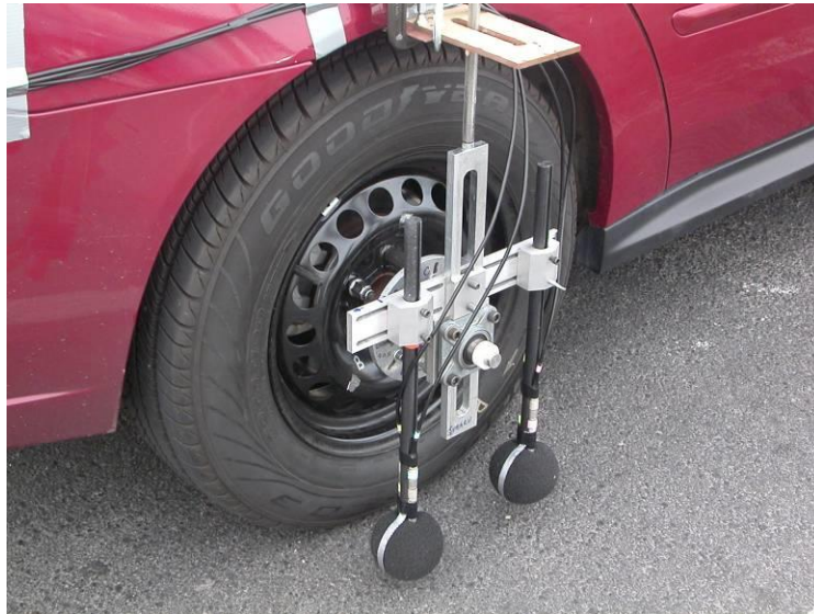
Figure 29. OBSI dual probe system and the SRTT.
