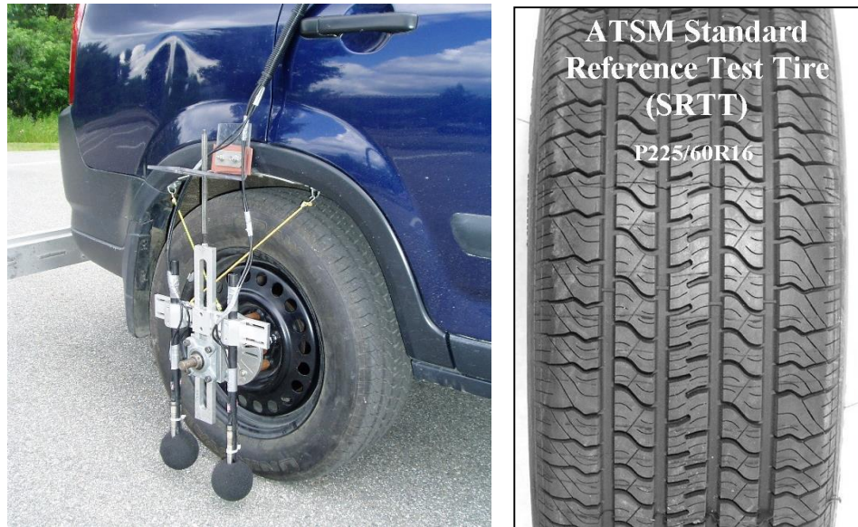
Figure 21. OBSI dual probe system and the SRTT.
