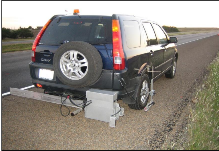
Figure 24. Laser profiler mounted behind the test vehicle.
