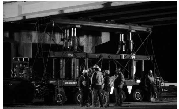
SPMTs are multi-axle computer controlled vehicles that can move in any horizontal direction and also have vertical lift.
