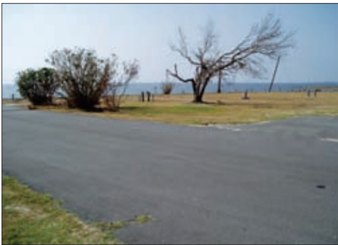
Figure 10. The site on the left is mapped Zone AE, and lies directly along the Gulf of Mexico shoreline. Limited obstructions to waves indicate the site could be classified as a Coastal A zone. The site on the right is over \frac{1}{2} mile from the Gulf shoreline, is mapped as Zone AE, and has a base flood stillwater level sufficient to support >1.5' wave heights – but obstructions to waves (e.g., trees and other buildings between the site and the shoreline) and distance from the source of flooding would indicate the area is not a Coastal A zone.
