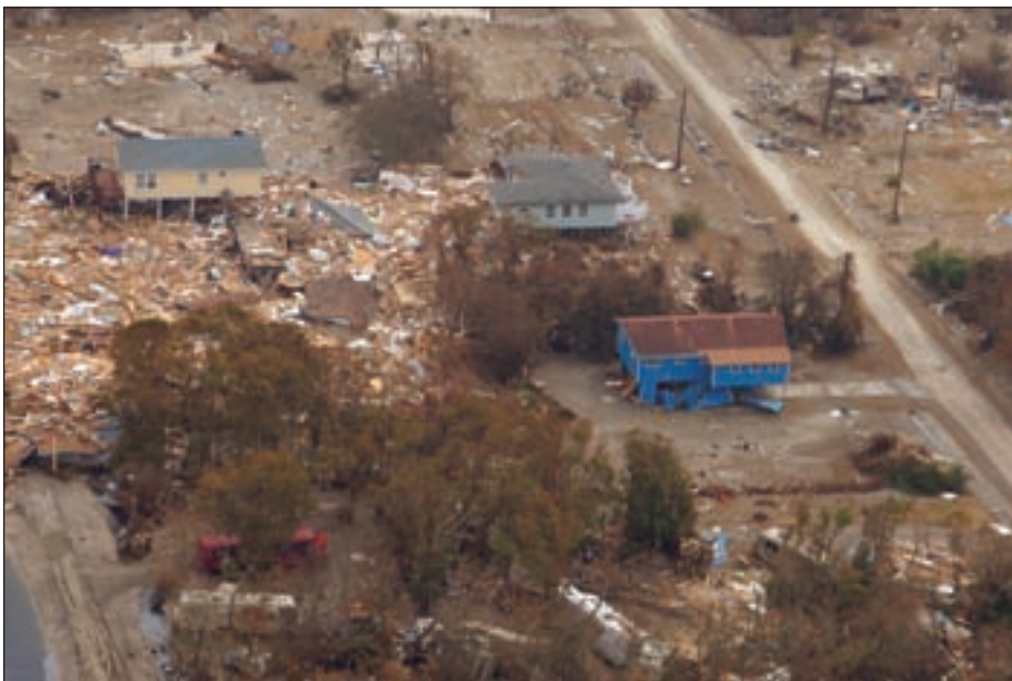
Figure 3-33. Roofs, walls, and other parts of destroyed houses washed landward to and inland of this location, approximately 1/2 mile from the Gulf shoreline of Bolivar Peninsula, TX
