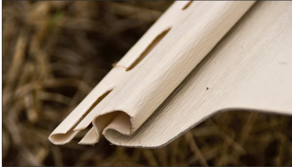
Figure 3-82. Vinyl siding rated for high wind has a double-layer nail hem
