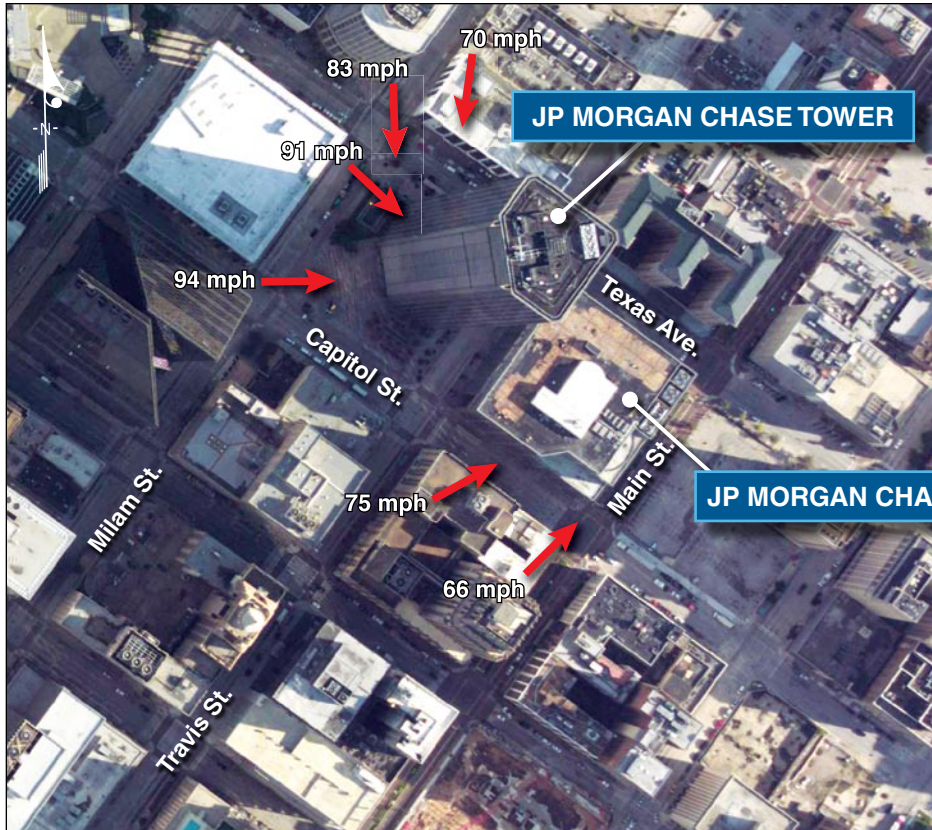
Figure 5-6. JP Morgan Chase Tower and JP Morgan Chase Center. The arrows show Hurricane Ike's primary wind directions (see text box) and maximum gust speed (for Exposure C at 33 feet above grade) for the given direction. 1
