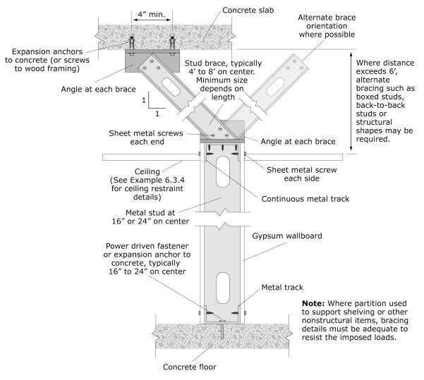
Figure 6.3.2.2-7 Partial height nonbearing stud wall (ER).
