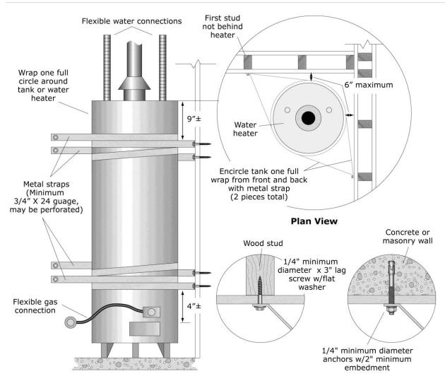
Figure 6.4.2.4–7 Water heater - corner installation (PR).
