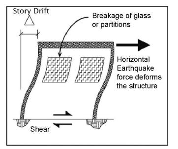
Figure 2.2.2-1 Nonstructural damage due to building deformation.
