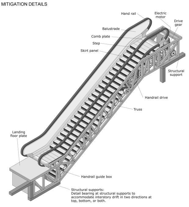
Figure 6.4.10.3-2 Schematic view of escalator (ER).
