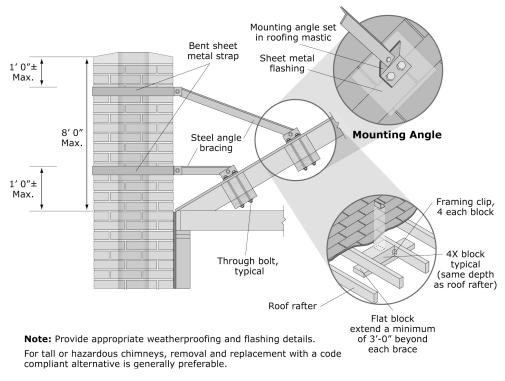
Figure 6.3.7.1-5 Unreinforced masonry chimney bracing (ER).
