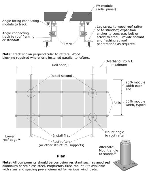
Figure 6.4.7.5-5 Typical details for flush-mounted photovoltaic power modules (ER).
