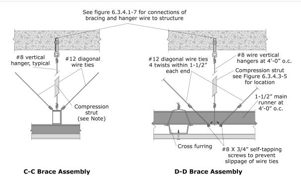
**Note:** Compression strut shall not replace hanger wire. Compresion strut consists of a steel section attached to main runner with 2 - #12 sheet metal screws and to structure with 2 - #12 screws to wood or 1/4" min. expansion anchor to concrete. Size of strut is dependent on distance between ceiling and structure ( $I/r \le 200$ ). A 1" diameter conduit can be used for up to 6', a 1-5/8" X 1-1/4" metal stud can be used for up to 10'. See figure 6.3.4.1-6 for example of bracing assembly.
