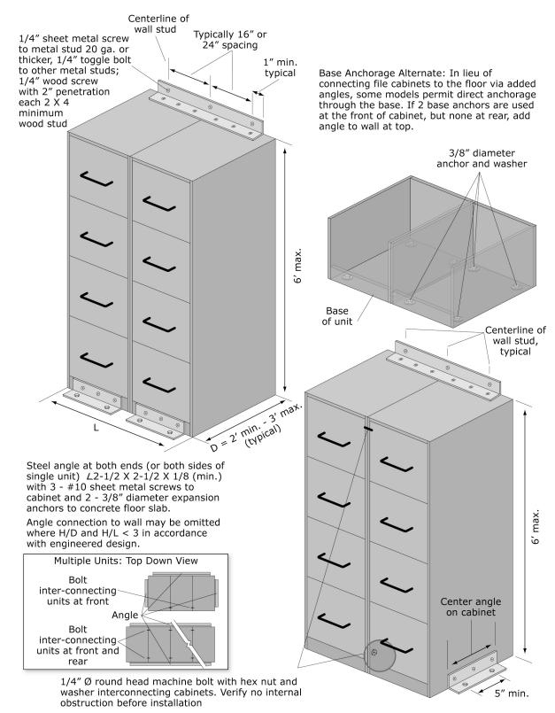
Figure 6.5.5.1-4 Wall-mounted file cabinets (NE).
