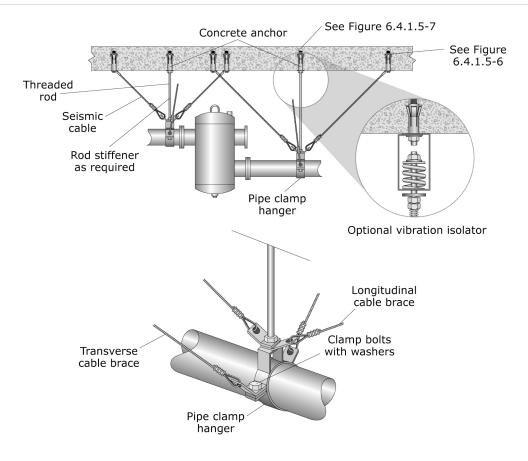
Figure 6.4.3.2–3 In-line valves and pumps (ER).
