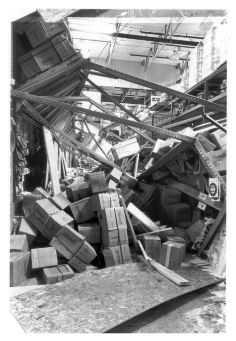
Figure 2.4.1-5 Damage to overloaded racks during the 1994 magnitude-6.7 Northridge Earthquake (FEMA 460, 2005).
