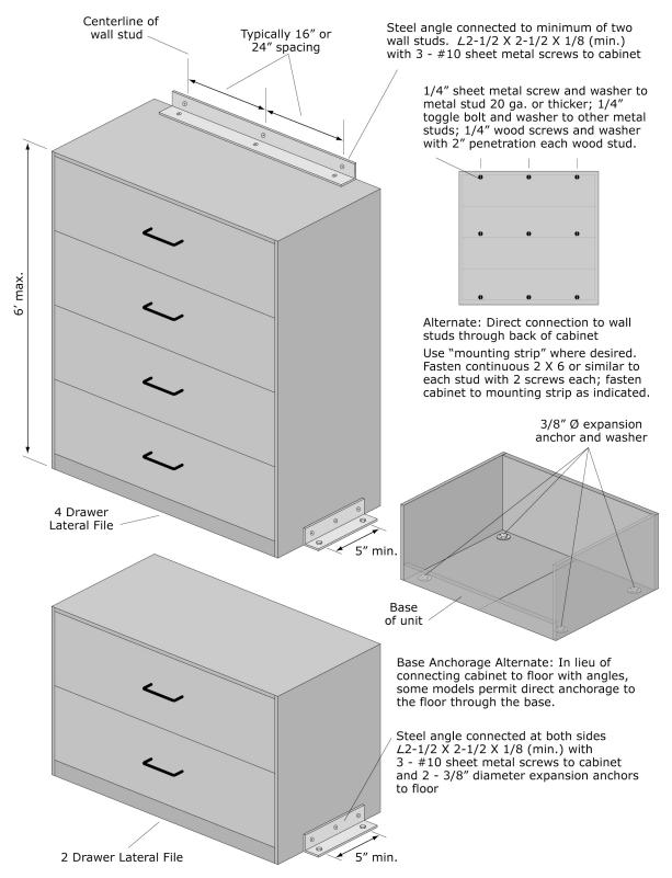
Figure 6.5.5.1-6 Wall-mounted and base-anchored lateral file cabinets (NE).
