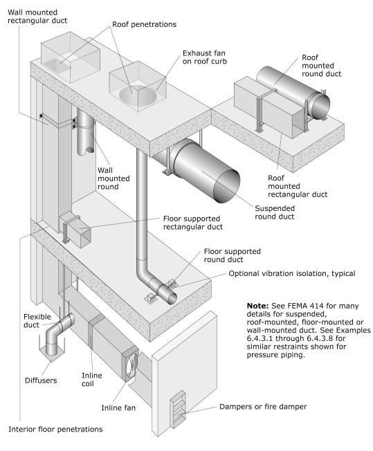
Figure 6.4.6.1–7 Overview of ductwork restraints (ER).
