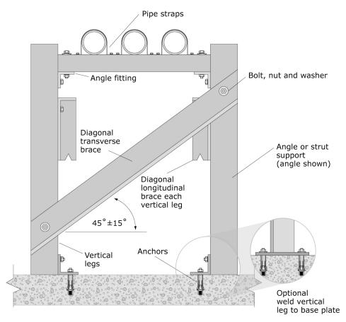
Figure 6.4.3.5-8 Floor-mounted pipe stand (steel shapes) (ER).
