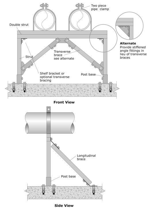
Figure 6.4.3.5-7 Floor-mounted pipe stand (strut frame) (ER).
