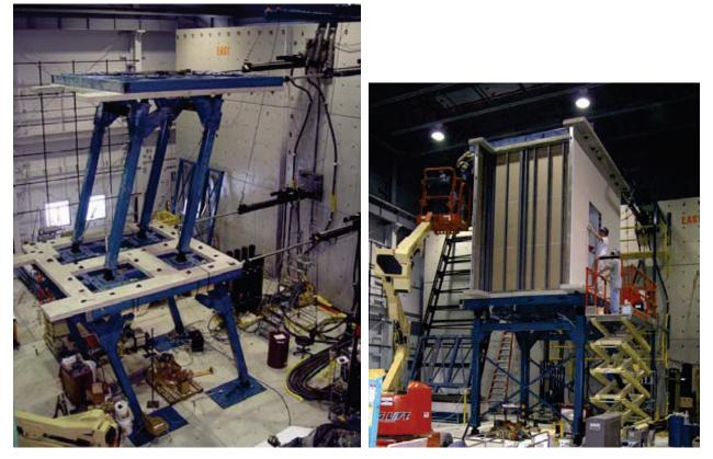
Figure 6.3.2.2-5 Two-story nonstructural component simulator at the University of Buffalo, SUNY shown at left. Preparation for dynamic testing of stud partitions for the NEES Nonstructural Project shown at right. Tests such as these improve understanding of the seismic behavior of nonstructural components (Photos courtesy of University of Buffalo, SUNY).
