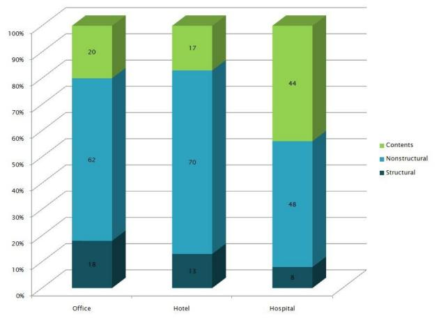
Figure 2.1.3-1 Typical investments in building construction.
