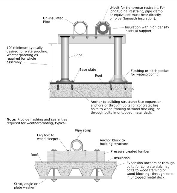
Figure 6.4.3.6-6 Roof-mounted pipe stand and sleeper anchored to slab (ER).
