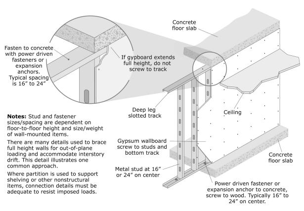
Figure 6.3.2.2-6 Full height nonbearing stud wall (ER).
