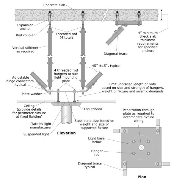
Figure 6.4.9.4-4 Details for supporting heavy light fixture directly from structure (ER).
