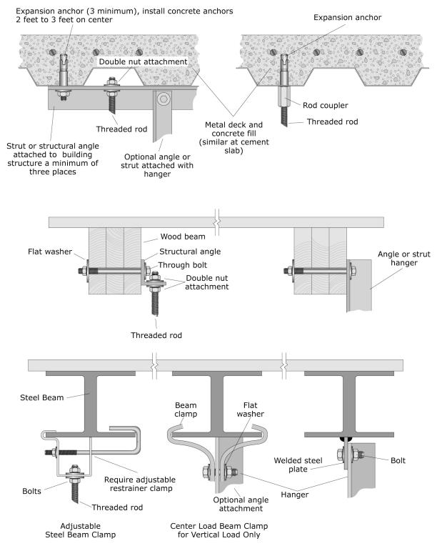
Figure 6.4.1.5–7 Hanger attachment details (ER).
