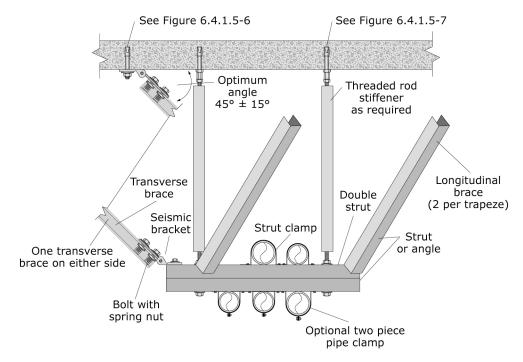
Figure 6.4.3.1-15 Rigid bracing - Trapeze supported piping (ER).
