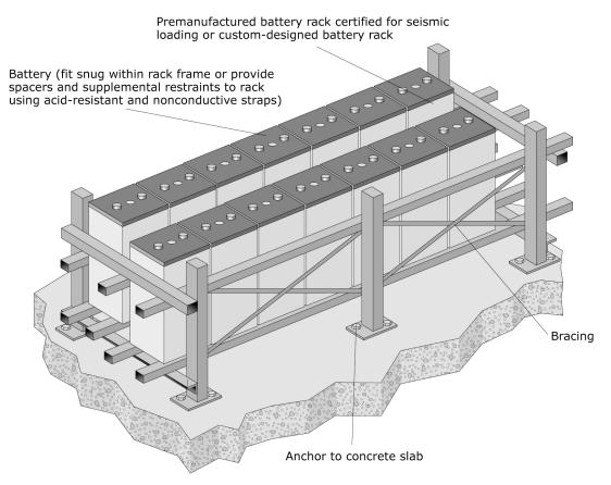
Figure 6.4.7.4-5 Batteries and rack (ER).
