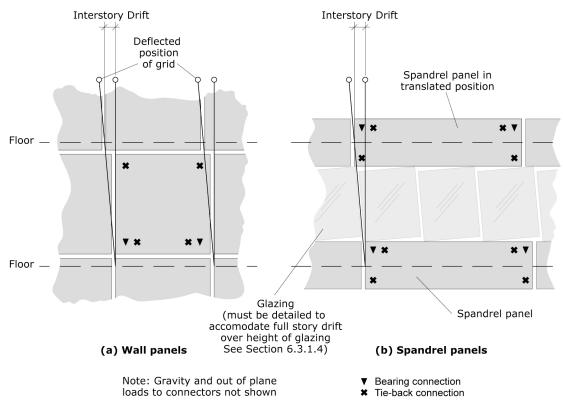
Figure 6.3.1.3-8c Low aspect ratio panels designed to accommodate seismic drift.
