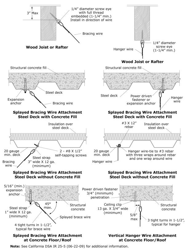
Figure 6.3.4.1-11 Suspension system for lay acoustic lay-in panel ceiling – overhead attachment details (PR).
