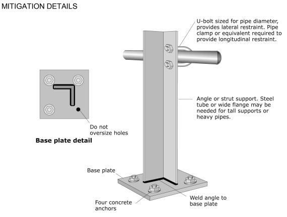
Figure 6.4.3.5-6 Floor-mounted single vertical pipe support (ER).
