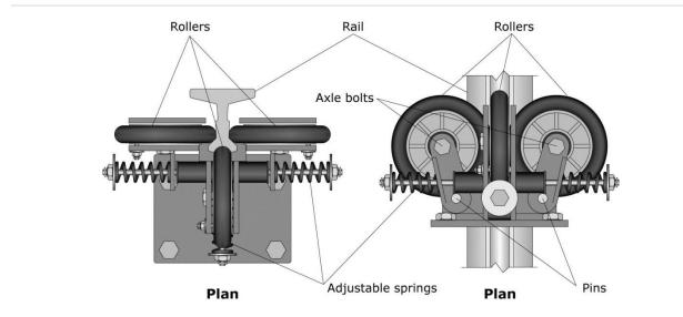
Figure 6.4.10.2-15 Spring loaded elevator guide with polyurethane rollers. Details of elevator guides vary from manufacturer to manufacturer, elevator load capacity, elevator speed, and whether used for guiding the car or counterweight.
