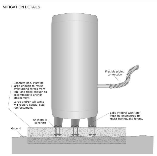
Figure 6.4.2.1–8 Vertical tank on legs (ER).
