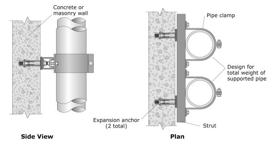
Figure 6.4.3.7-4 Surface-mount to structural wall (ER).
