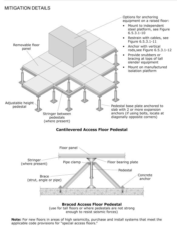
Figure 6.5.3.1-9 Equipment mounted on access floor (ER).
