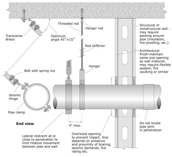
Figure 6.4.3.8-7 Wall penetration (ER).
