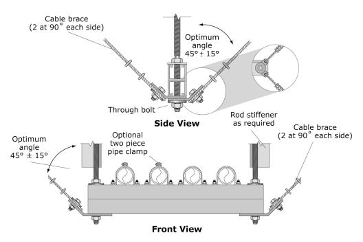
Figure 6.4.3.1-16 Cable bracing - Trapeze supported piping (ER).
