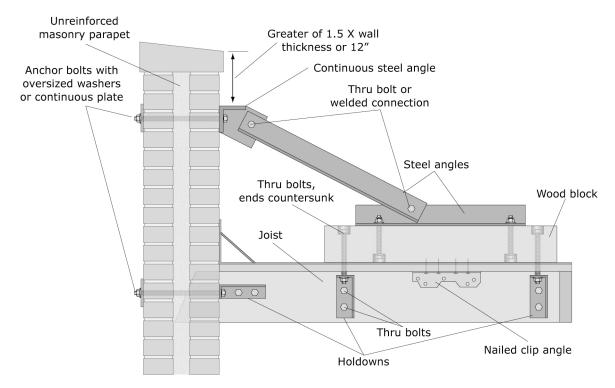
**Note:** Typical brace configuration shown; parapet and roof conditions may vary widely. Provide appropriate weatherproofing and flashing details.
