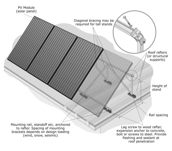
**Note:** All components should be corrosion resistant such as anodized aluminum or stainless steel. Proprietary tilt-up kits available with sizes and spacing pre-engineered for various wind loads.
