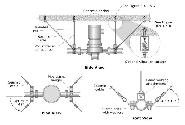
Figure 6.4.3.2–2 In-line valves and pumps (ER).
