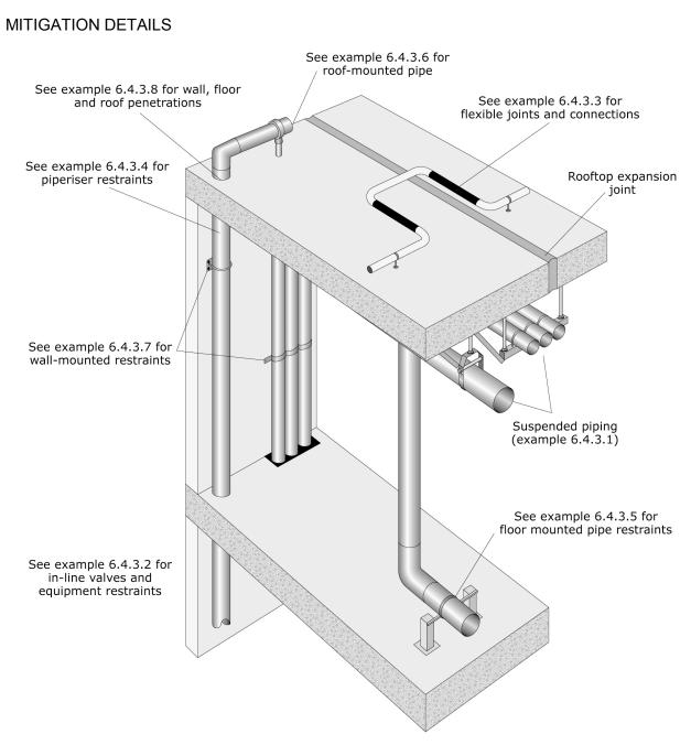
Figure 6.4.3.1-10 Schematic of seismic restraint conditions for piping (ER)
