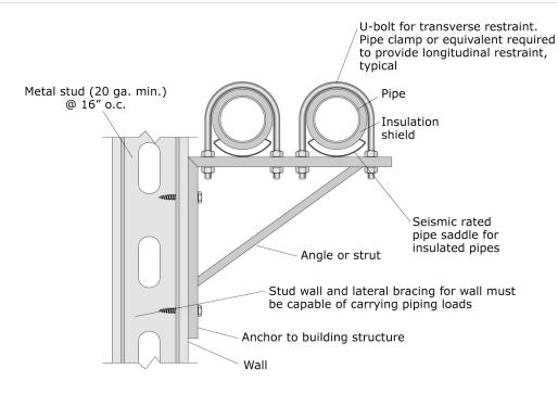
Figure 6.4.3.7-7 Wall-mount to stud wall with pre-manufactured brackets (ER).
