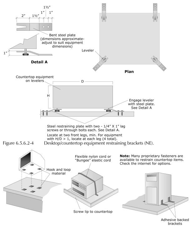
Figure 6.5.6.2-5 Desktop/countertop equipment restraining straps (NE).
