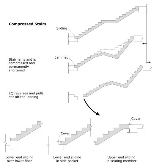
Figure 6.3.8.1-6 Figure showing how inadequate sliding surface can compress and then drop precast stair sections.
