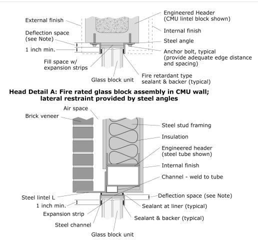
Head Detail B: Non-rated glass block assembly in steel stud wall with brick veneer; lateral restraint provided by steel channel
