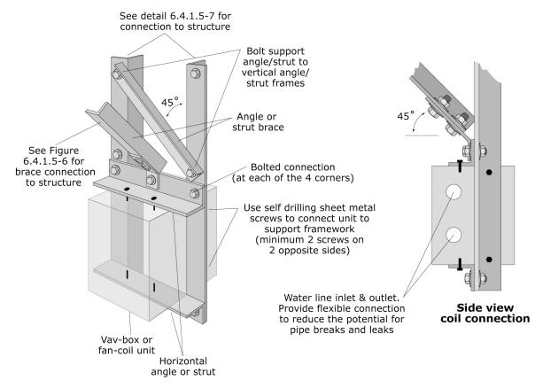
Figure 6.4.1.5-5 HVAC equipment suspended in-line with ductwork (ER).
