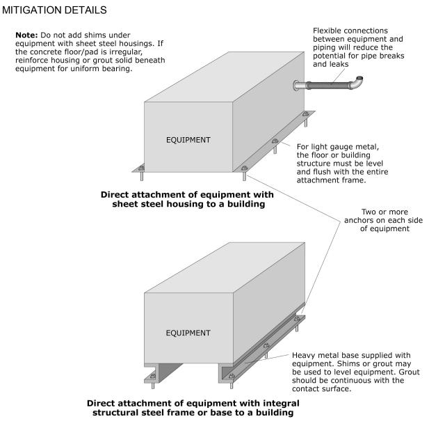
Figure 6.4.1.1-6 Floor-mounted equipment – anchored through integral base (ER).
