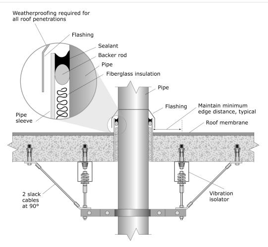
Figure 6.4.3.4-8 Roof penetration with vibration isolation (ER).
