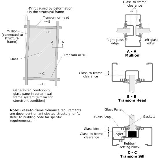
Figure 6.3.1.4-7 Glazed exterior wall system (ER).
