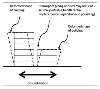
Figure 2.2.3-1 Nonstructural damage due to separation and pounding.
