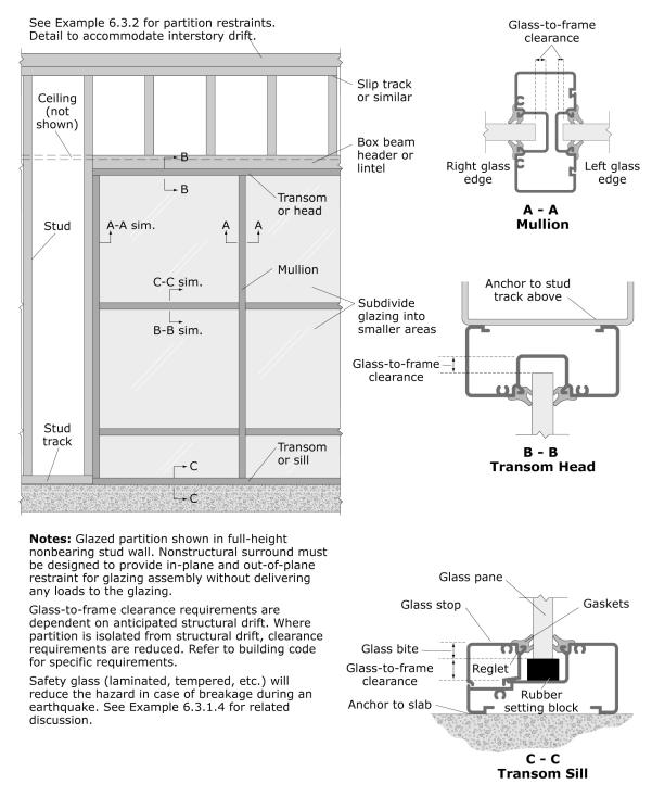
Figure 6.3.2.3-6 Details for full-height glazed partition (ER).
