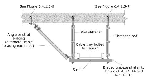
Figure 6.4.8.1-5 Cable tray on braced trapeze (ER).
