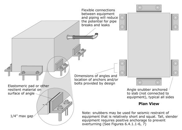
Figure 6.4.1.1-7 Floor-mounted equipment – restrained with snubbers.
