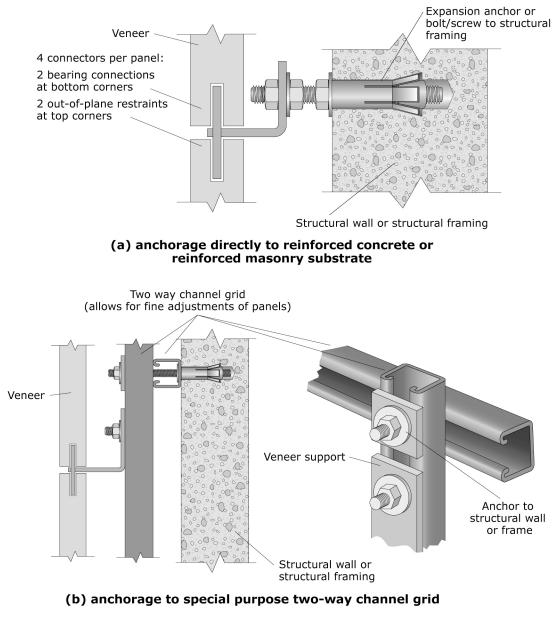
Figure 6.3.3.1-3 Detail for anchored interior veneer (ER).
