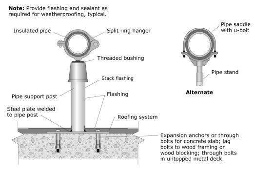
Figure 6.4.3.6-5 Roof-mounted single vertical pipe support (ER).
