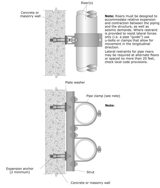
Figure 6.4.3.4-5 Wall-mounted pipe riser restraint/support (ER).
