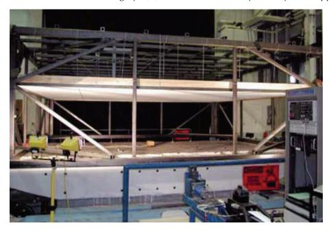
Figure 6.3.4.1-7 Shake table testing of a proprietary suspended acoustic lay-in tile ceiling at MCEER (Photo courtesy of University of Buffalo, SUNY). Additional testing of these systems will help improve our understanding of their failure modes and help inform the design of more resilient systems.
