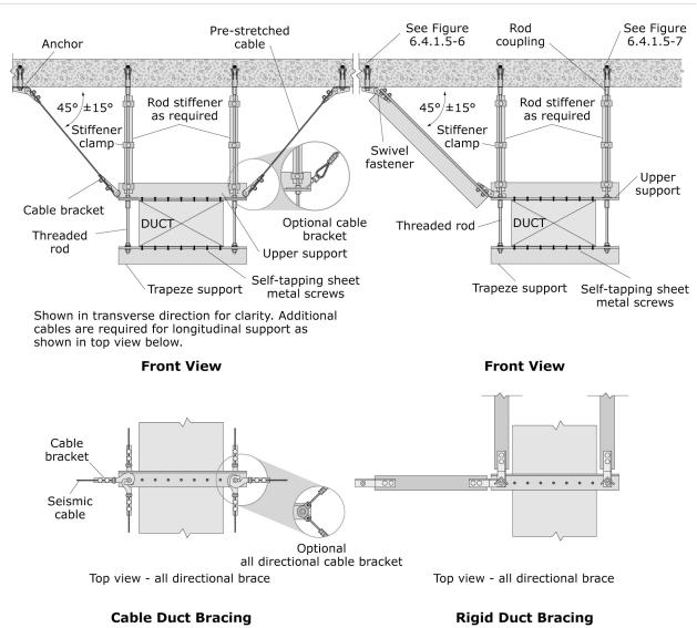
Figure 6.4.6.1–8 Suspended ductwork (ER).
