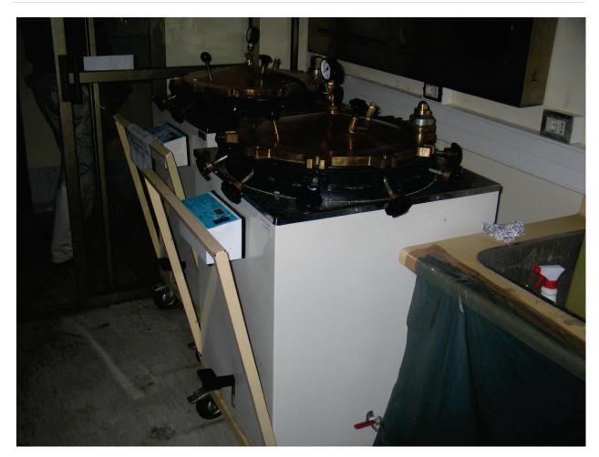
Figure 6.5.5.3-3 Equipment on wheels did well during the 2010 magnitude-8.8 Chile Earthquake; there were no reported injuries or examples of overturning related to equipment mounted on wheels. Centrifuges on wheels shown in photo (Photo and information courtesy of Bill Holmes, Rutherford & Chekene).
