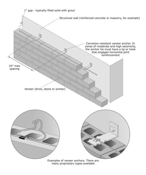
Figure 6.3.1.2-5 Anchored veneer (ER).
