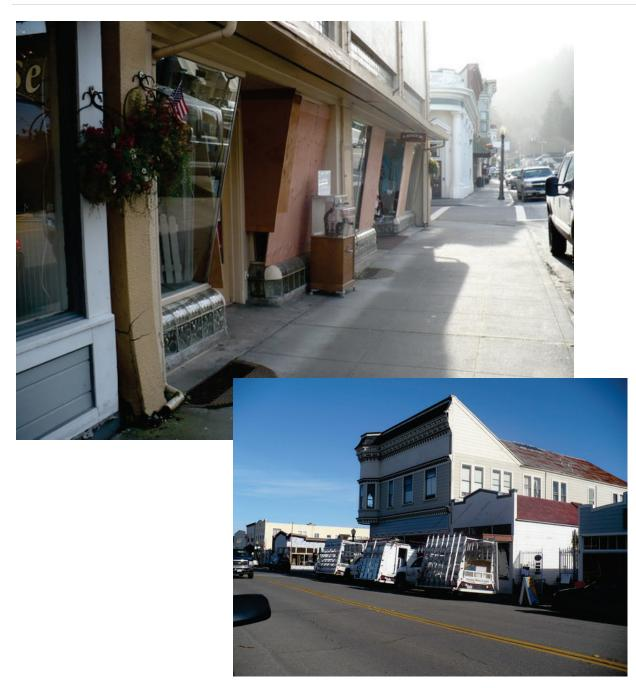
Figure 6.3.1.4-2 Scenes in Ferndale, California following the 2010 magnitude-6.5 Eureka Earthquake. 50% of the glazing on Main Street was cracked (Photos courtesy of Bret Lizundia, Rutherford & Chekene). Available at: http://www.fema.gov/earthquake-publications/fema-e-74-reducing-risks-nonstructural-earthquake-damage Last Modified: December 2012
