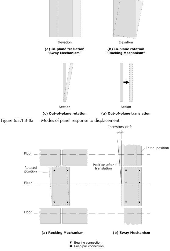
Figure 6.3.1.3-8b Tall and narrow panels designed to accommodate seismic drift.
