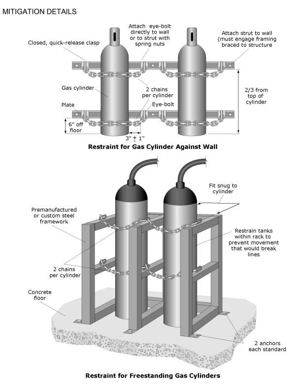
Figure 6.4.2.3–8 Compressed gas cylinders (ER).
