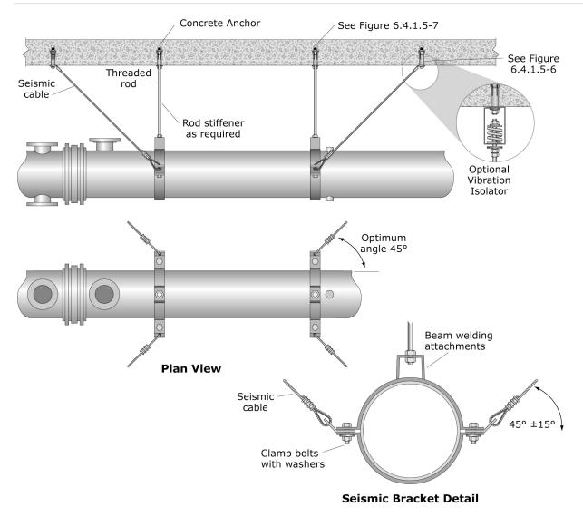
Figure 6.4.3.2–4 In-line valves and pumps (ER).
