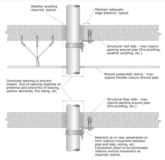
Figure 6.4.3.8-8 Floor or roof penetration (ER).
