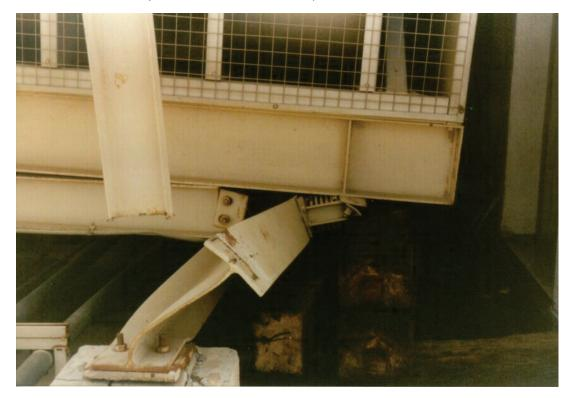
Figure 6.4.1.3-3 Failure of an entire support assembly including vibration isolators (Photo courtesy of Mason Industries).
