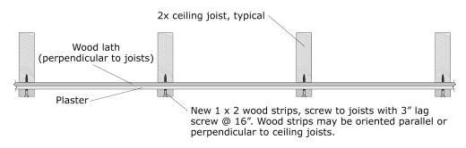
Figure 6.3.4.2-9 Retrofit detail for existing lath and plaster (NE).
