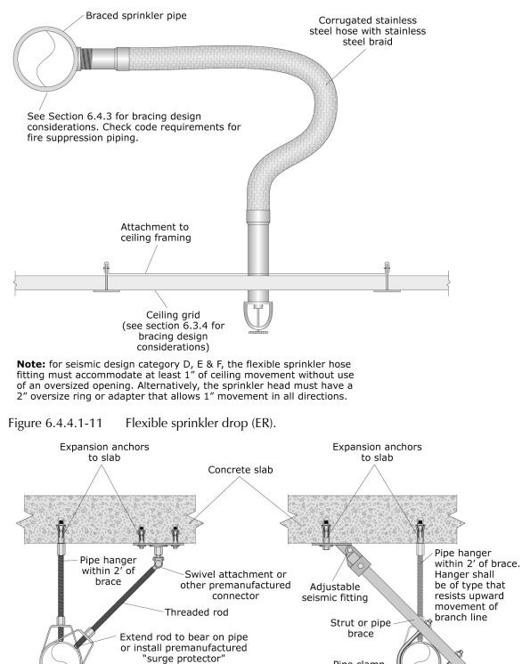
Figure 6.4.4.1–12 End of line restraint (ER).
