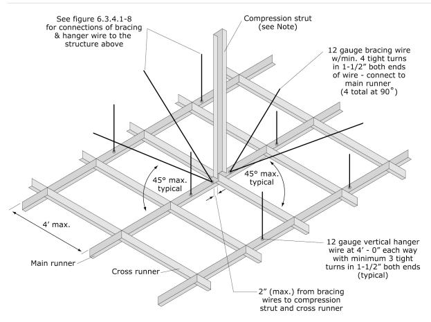
**Note:** Compression strut shall not replace hanger wire. Compression strut consists of a steel section attached to main runner with 2 - #12 sheet metal screws and to structure with 2 - #12 screws to wood or 1/4" min. expansion anchor to structure. Size of strut is dependent on distance between ceiling and structure ( $I/r \le 200$ ). A 1" diameter conduit can be used for up to 6', a 1-5/8" X 1-1/4" metal stud can be used for up to 10'
