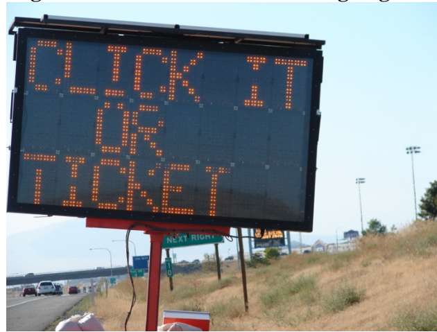
Figure 3. Portable variable message sign
