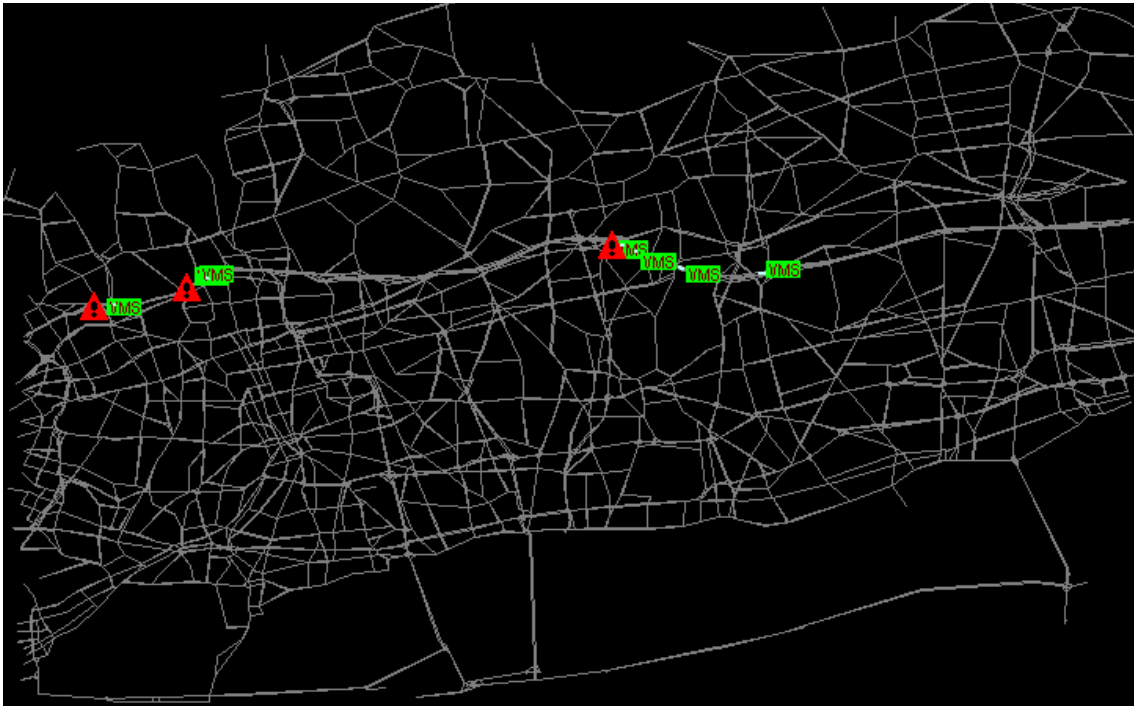
b) Detour signs are activated at selected exits along the adjacent upstream segment
