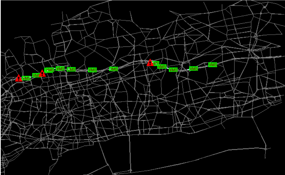
a) Detour signs are activated at every exit along the adjacent upstream segment
