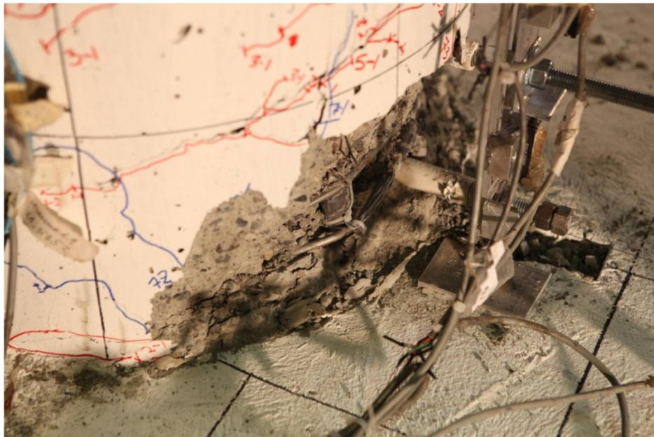
Figure 125. Photo. Specimen SF-1: first noticeable bar buckling was the N-NW bar in cycle 9-2 (+7.40/-7.40 target drift ratio).
