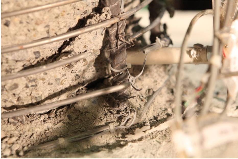
Figure 126. Photo. Specimen SF-1: N-NE bar fractured first when the column was loaded to peak in cycle 10-2 (+10.65/-10.65 target drift ratio).
