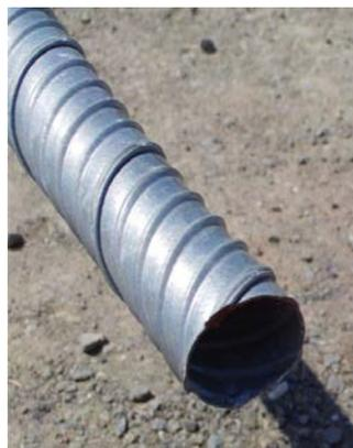
Figure 121. Photo. Corrugated metal duct used in test specimens.
