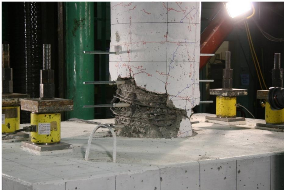
Figure 135. Photo. Specimen SF-2: damage after the cyclic testing.
