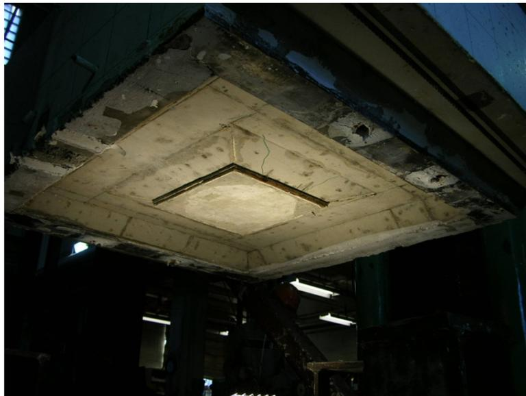
Figure 63. Photo. Specimen SF-2 after axial load of 817 kips.
