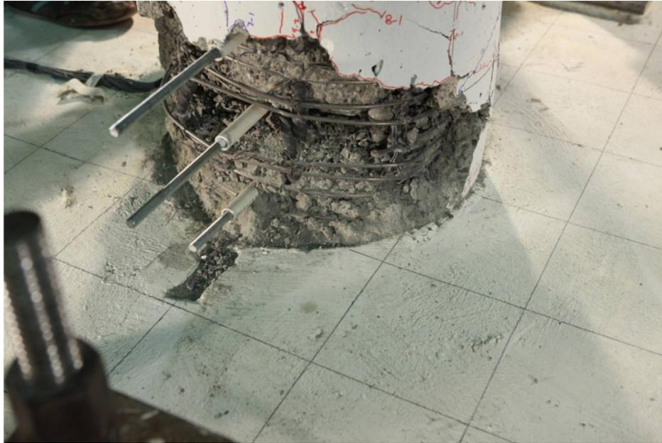
Figure 136. Photo. Specimen SF-2: no damage to the footing was observed after the cyclic testing.
