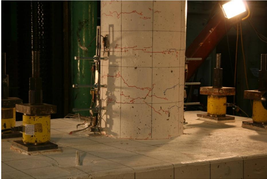
Figure 122. Photo. Specimen SF-1 flexural cracks after cycle 4-1 (+1.00/-1.00 target drift ratio).
