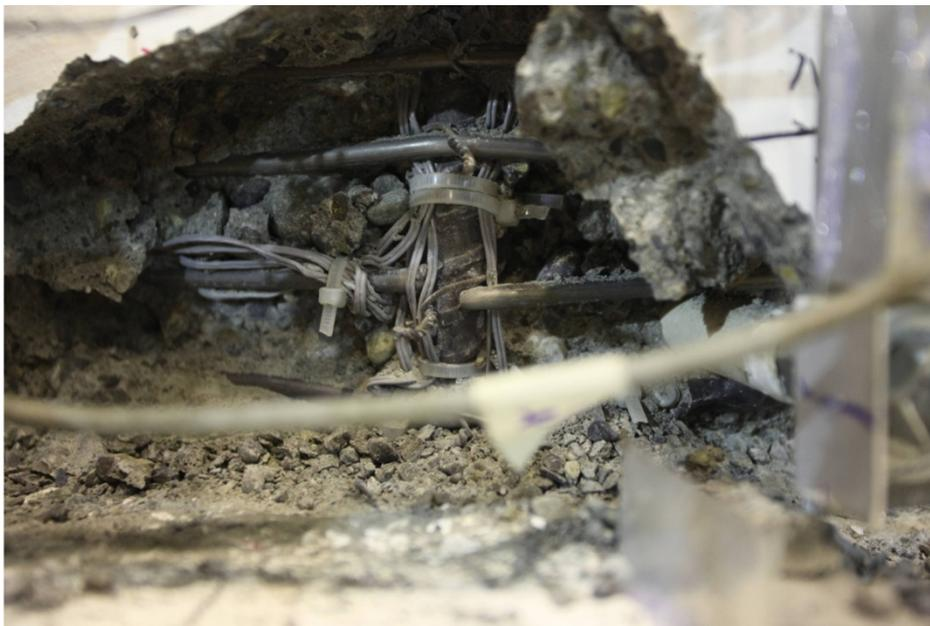
Figure 149. Photo. Specimen SF-3: fracture of transverse reinforcement in cycle 10-1 (+8.87/-8.87 target drift ratio).
