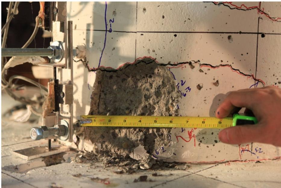
Figure 131. Photo. Specimen SF-2: first significant spalling at cycle 7-1 (+2.97/-2.97 target drift ratio).
