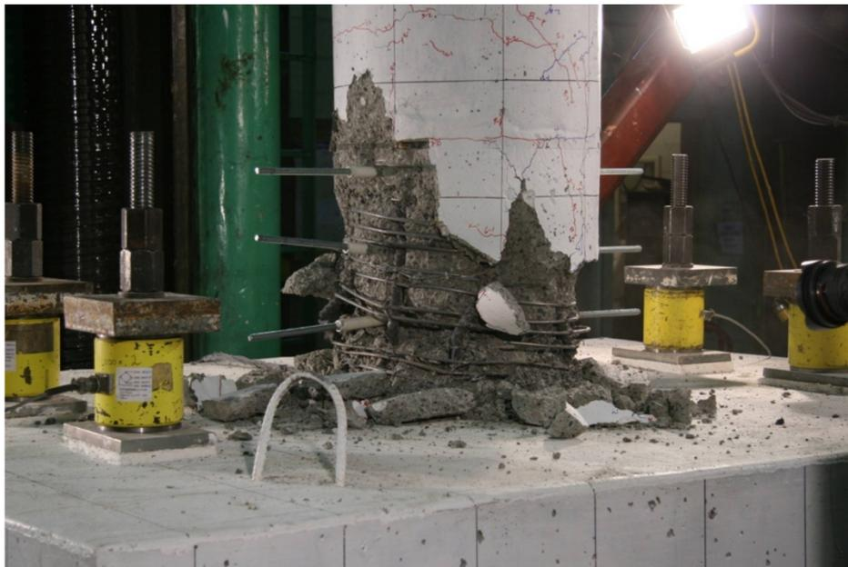
Figure 137. Photo. Specimen SF-2: damage the end of testing. The column crushed after application of vertical load of 819.5 kips.
