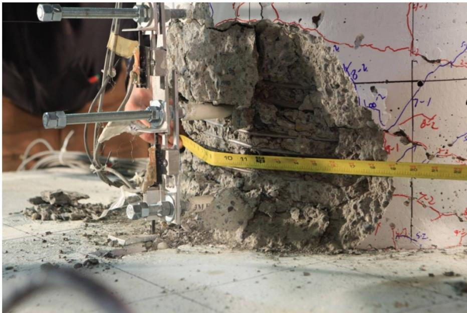
Figure 133. Photo. Specimen SF-2: first noticeable bar buckling was the N-NW bar in cycle 9-3 (+7.40/-7.40 target drift ratio).
