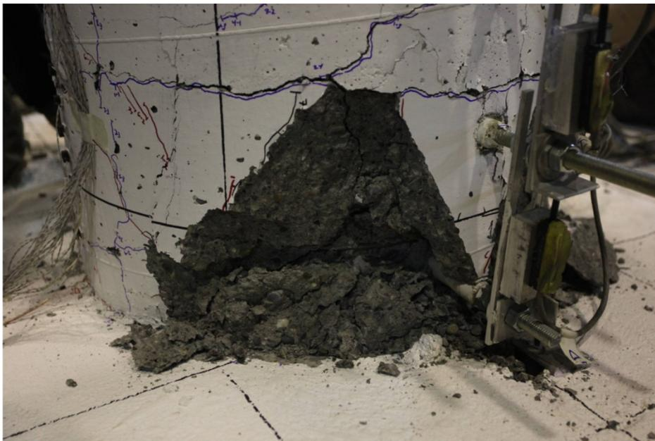
Figure 147. Photo. Specimen SF-3: transverse steel exposed in cycle 9-3 (+7.40/-7.40 target drift ratio).
