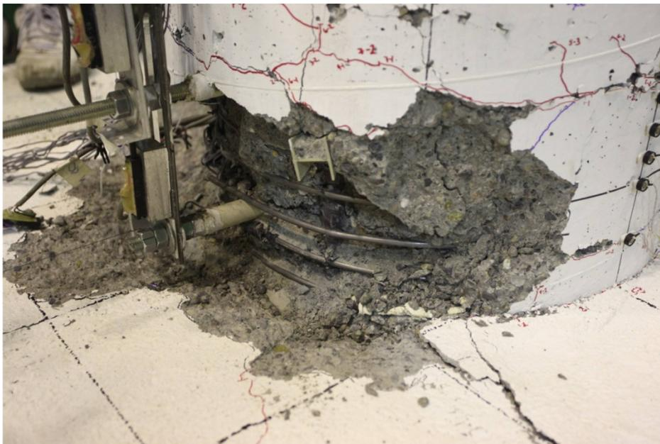
Figure 151. Photo. Specimen SF-3: major cracks in the concrete core in cycle 10-2 (+10.65/-10.65 target drift ratio).
