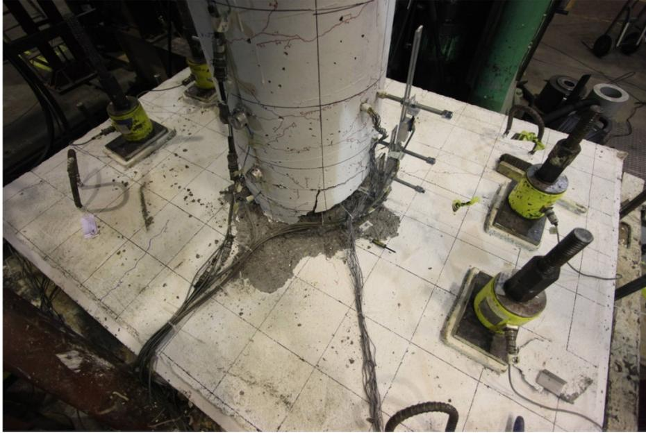
Figure 152. Photo. Specimen SF-3: condition of specimen just before last cycle.
