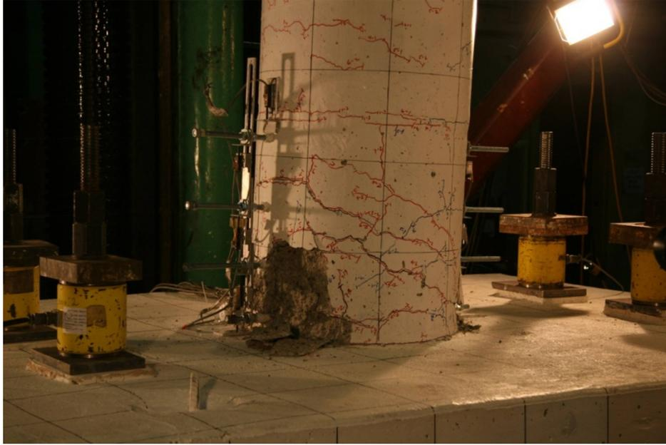
Figure 124. Photo. Specimen SF-1: plastic hinge became more pronounced in subsequent cycles. Photo taken during cycle 8-1 (+4.28/-4.28 target drift ratio).
