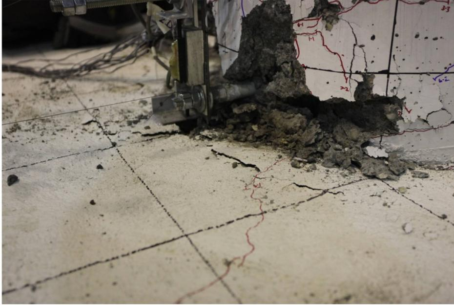
Figure 146. Photo. Specimen SF-3: first footing spalling in cycle 9-2 (+7.40/-7.40 target drift ratio).
