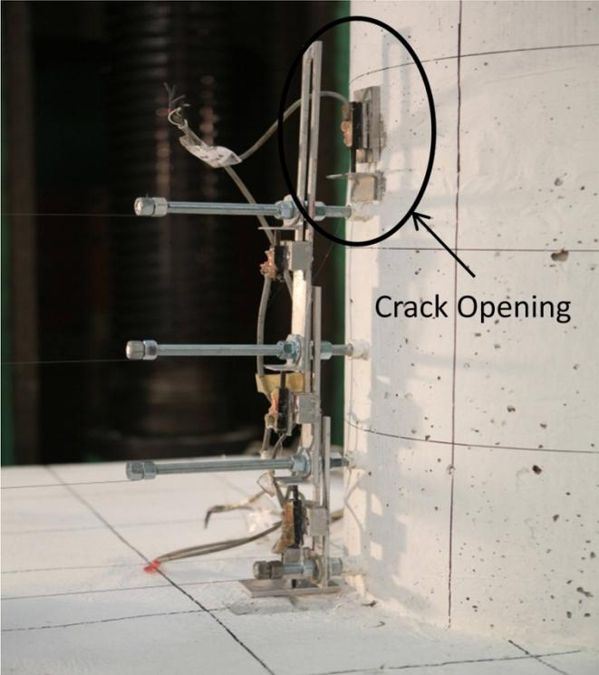
Figure 38. Photo. Crack opening measurement pot.
