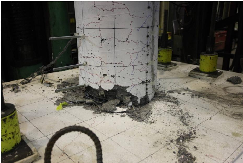
Figure 153. Photo. Specimen SF-3: column after punching through in last cycle (cycle 10-3, +10.65/-10.65 target drift ratio).
