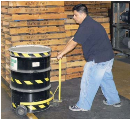
This three-wheel cart transports but does not lift drums.
