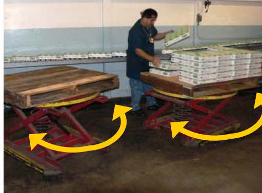
Turntable on a load leveler
