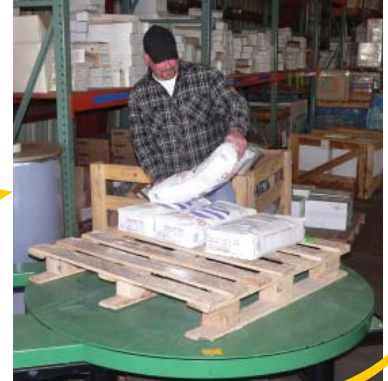
A fixed-height turntable for pallets with short low stacks.
