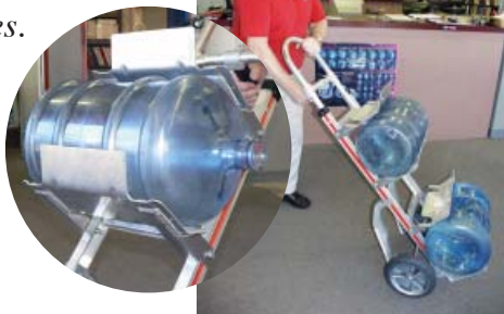
Two-wheel hand trucks work well for transporting bottles or cylinders over short distances.
