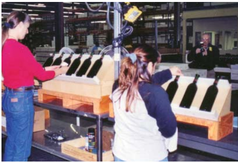
Provide variable-height work surfaces.
