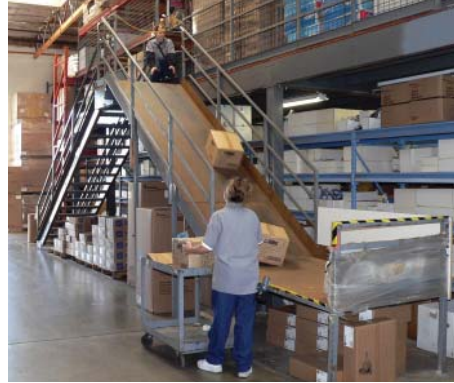
Use slides or chutes to do the work if containers are always moving in one direction.
