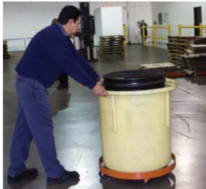
The drum must be set down into this dolly.
