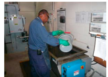
Solvent must be replaced before reaching the threshold for hazardous waste.
