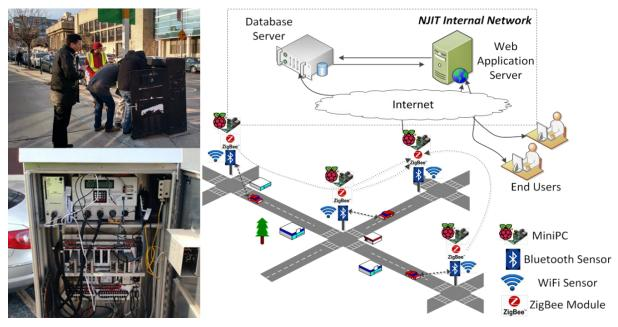
Figure 7. Newark – NJIT Corridor Instrumentation Pilot
