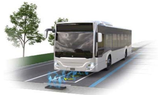
Wireless is one of several charging options Denver is exploring. Image courtesy of Josh Bauer, NREL.
