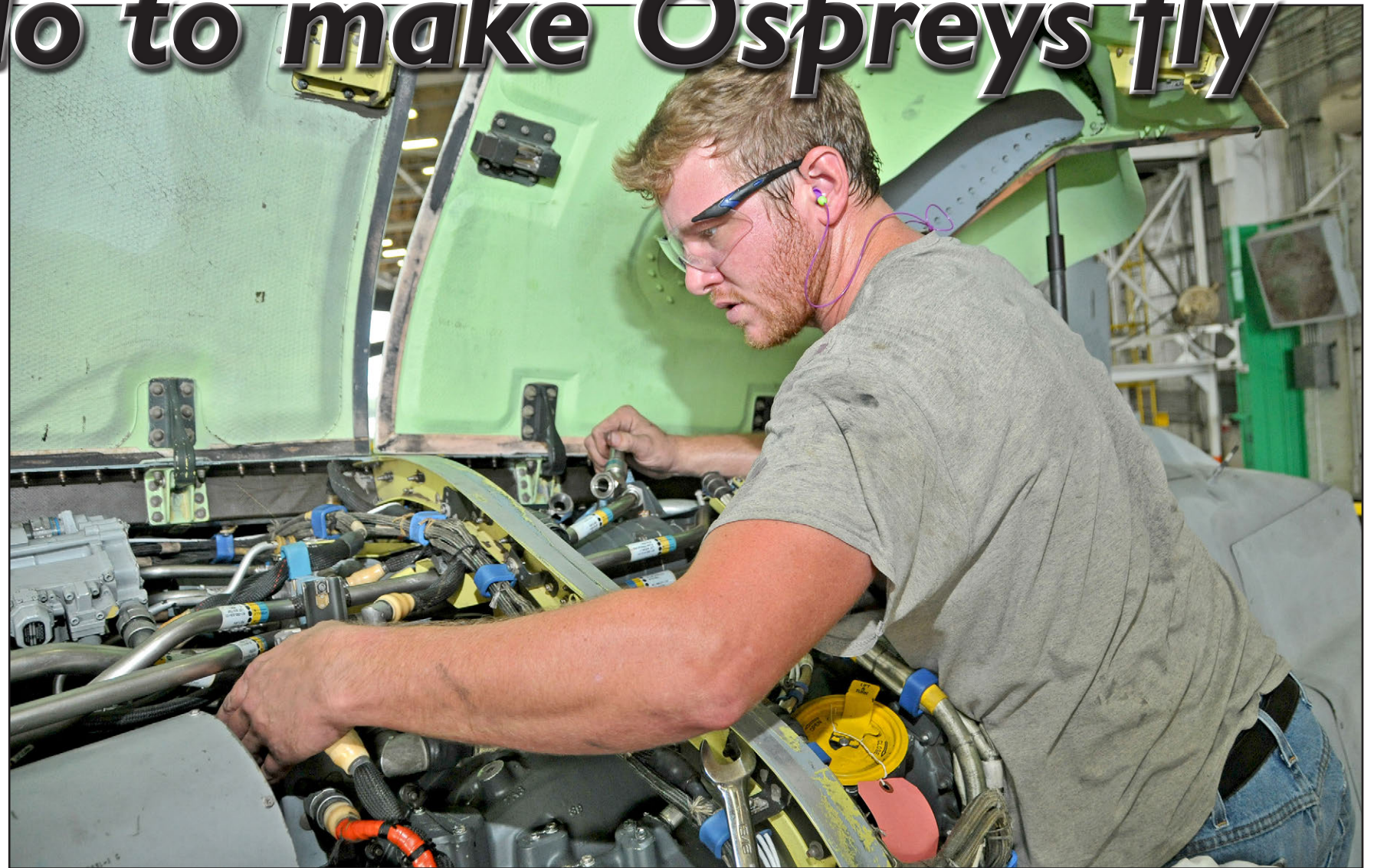
Frederick Ellis, aircraft mechanic, navigates the configuration of lines and other components to remove a hydraulic (system 1) line from a V-22 rotor wing Oct. 5 in Fleet Readiness Center East Building 137, Hangar 1.
