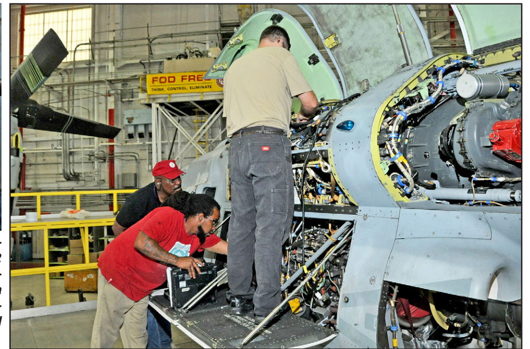
Frederick Ellis, aircraft mechanic, navigates the configuration of lines and other components to remove a hydraulic (system 1) line from a V-22 rotor wing Oct. 5 in Fleet Readiness Center East Building 137, Hangar 1.
