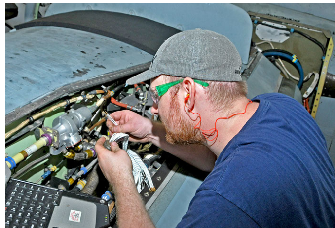
Chris Zeman, aircraft electrician, works to pin a connector to replace a damaged wire harness on a V-22 aircraft Oct. 5. Photo right: Jerry Besier, aircraft electrician, works up high to run a new wing harness in a nacelle, while Aircraft Workers Walter Bryant and Coboros Davis inspect the nacelle, according to technical manuals, to ensure the accuracy of part numbers.
