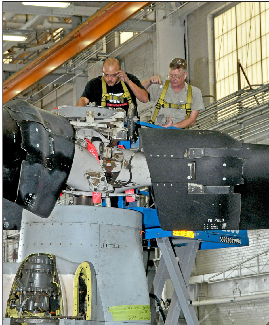
Frederick Ellis, aircraft mechanic, navigates the configuration of lines and other components to remove a hydraulic (system 1) line from a V-22 rotor wing Oct. 5 in Fleet Readiness Center East Building 137, Hangar 1.
