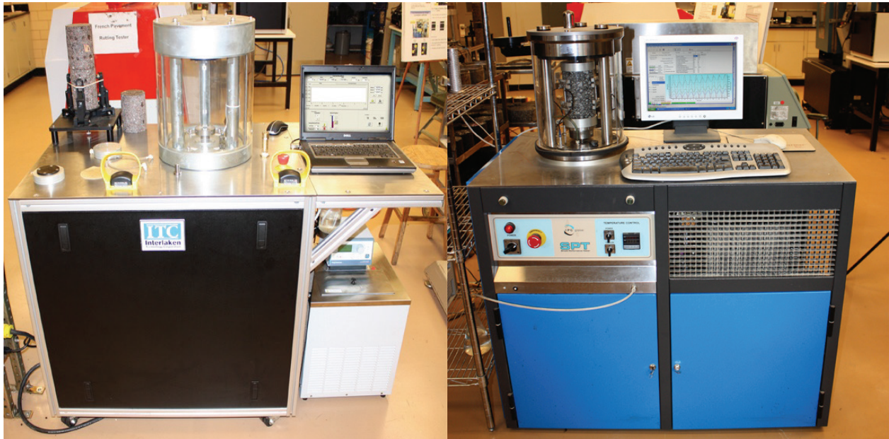
Figure 1. Photographs of AMPT Equipment by Interlaken Technology Corporation (left) and IPC Global (right).
