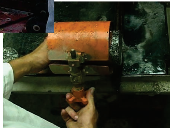
Figure 3. Major Steps in AMPT Test Specimen Preparation.
