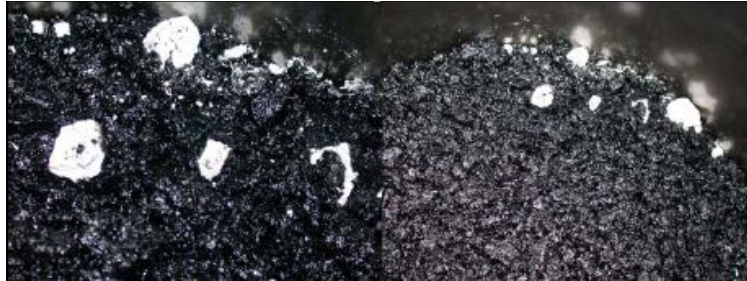
Figure 20. Photo. Characteristic lime nuggets indicating less than desired uniform mixing.
