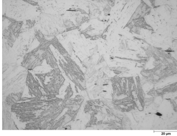
Figure 15. Photo. Microstructure of 9Cr plate from heat 67-V1-68 in the as-normalized condition: 500X.
