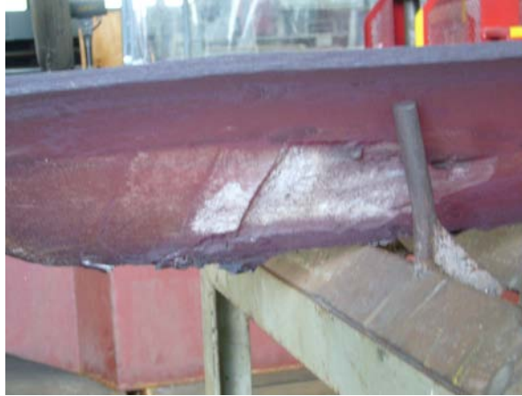
Figure 11. Photo. Heat 67-V1-79 after hot rolling and showing scab.
