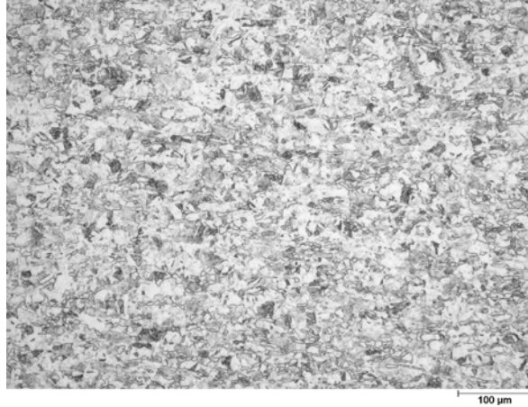
Figure 12. Photo. Microstructure of 11Cr plate from heat 67-V1-77 in the as-normalized condition: 100X.
