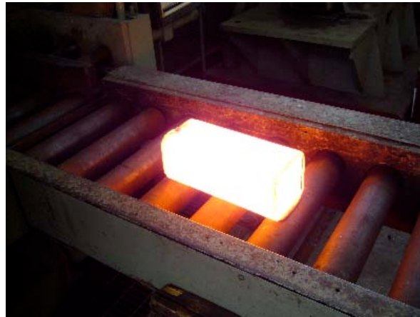
Figure 8. Photo. Heat 67-V1-83 being hot rolled prior to first pass.
