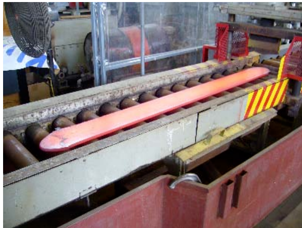
Figure 9. Photo. Heat 67-V1-83 being hot rolled after last pass.
