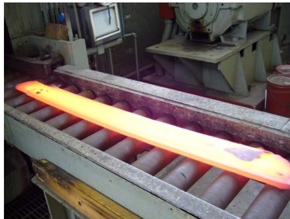
Figure 10. Photo. Heat 67-V1-79 being hot rolled and showing scab.
