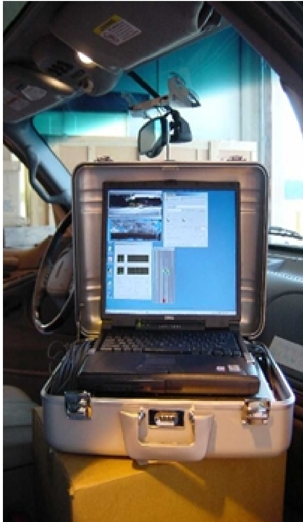
Figure 7. Photo. In-vehicle camera sensor and a portable briefcase processing system.
