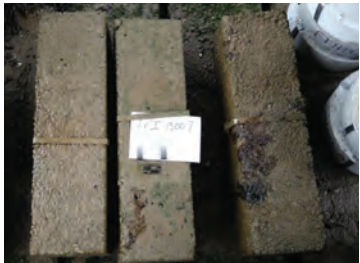
Figure 19. Slag geopolymer beams after 1 year of exposure at Treat Island.
