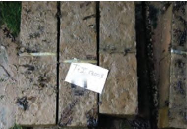
Figure 17. Fly ash geopolymer beams after 1 year of exposure at Treat Island.
