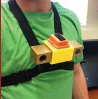
A chest-mounted stereo camera and inertial measurement unit form part of Auburn University's pedestrian navigation system.
