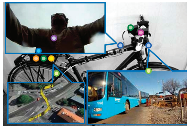
Figure 1. An instrumented traditional bicycle.
