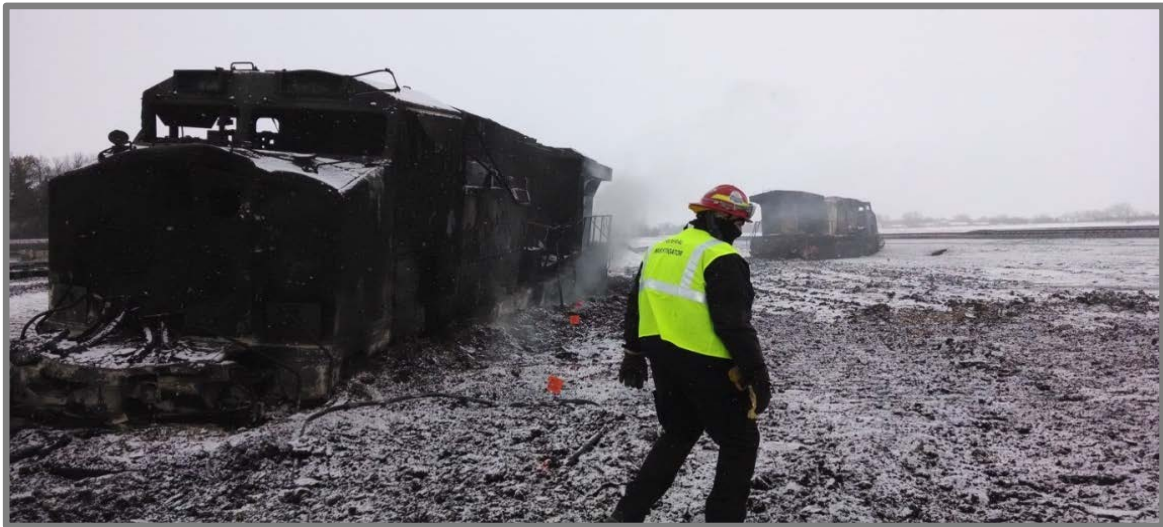
An oil train derailment near Casselton, N.D. hastens an investigator from PHMSA’s Central Region to the scene of this December 2013 incident to conduct damage assessment, shed light on the crashworthiness of the DOT 111 rail cars, while also sampling the crude oil aboard them. Photo by PHMSA Central Region.
