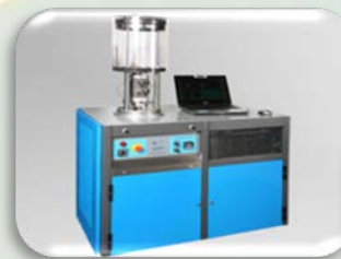
Mixture Cracking Evaluated with the AMPT Cyclic Fatigue Test
