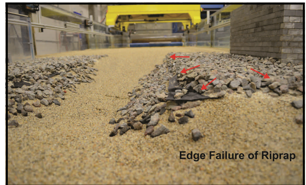
Physical Modeling results showing observed edge failure of the countermeasure.
