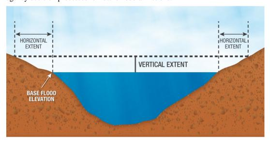
EO 11988 currently uses the base floodplain to determine the vertical elevation and floodplain boundary. The FFRMS increases both the vertical elevation and the corresponding area of the floodplain to which the FFRMS applies.
