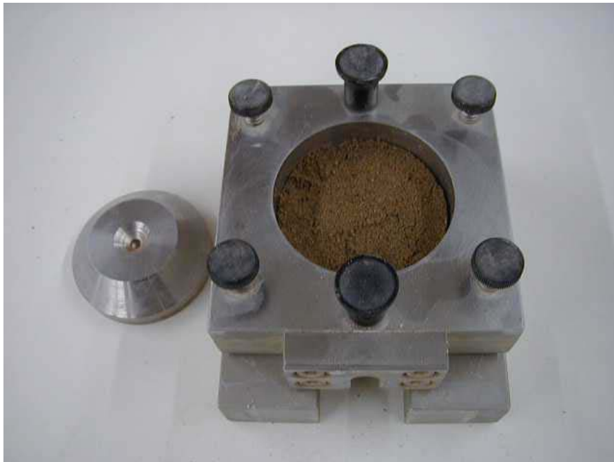
Figure 29. Direct shear testing box (photograph courtesy of GeoTesting Express).
