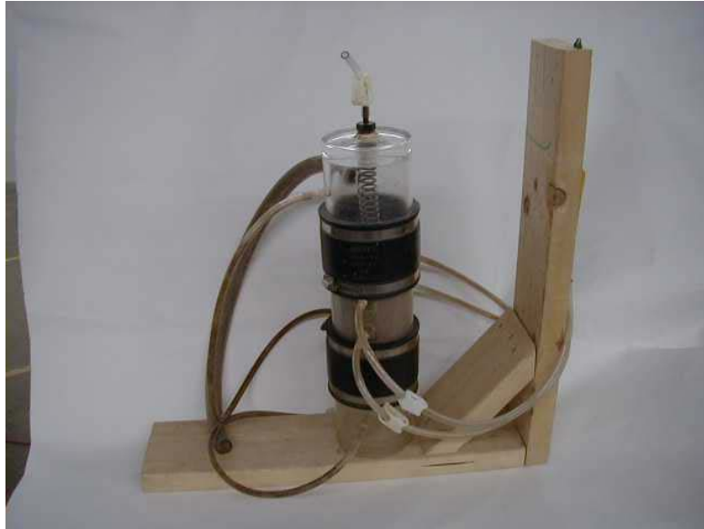
Figure 31. Rigid wall permeameter (photograph courtesy of GeoTesting Express).
