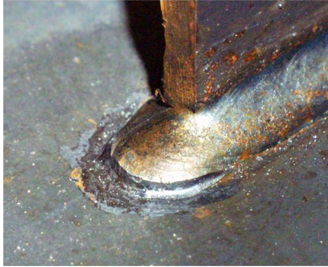
Figure 16. Photo. A peened weld toe, note the geometry and luster change at the weld toe.
