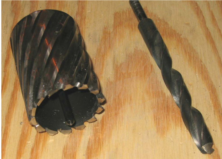
Figure 22. Photo. Annular cutter (left). Twist bit (right).
