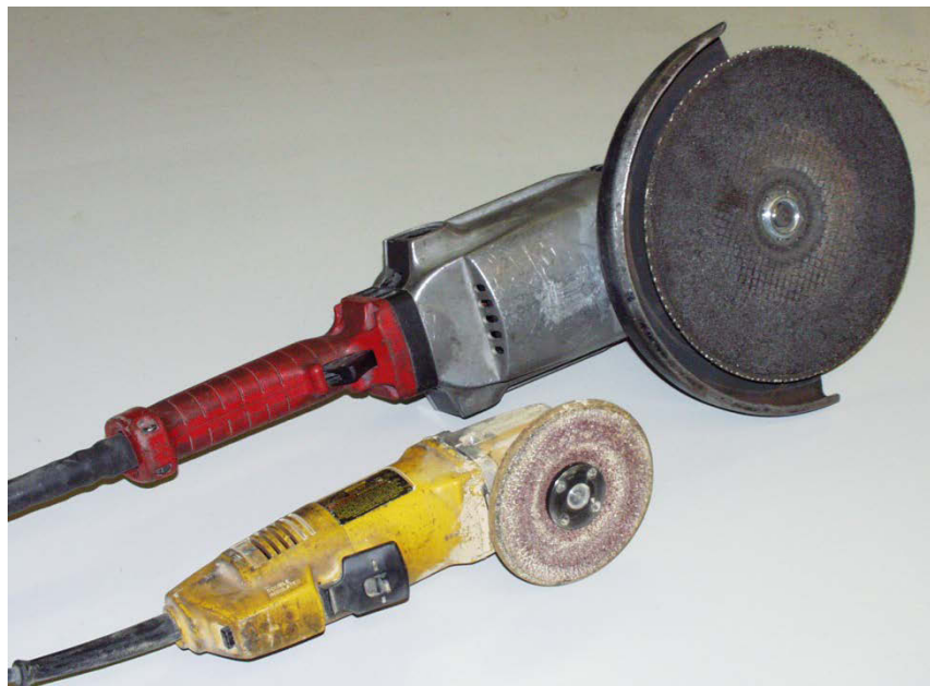
Figure 12. Photo. Typical disc grinders.
