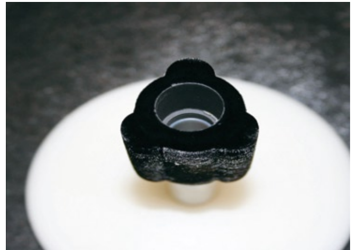
Shaped cathode for the relativistic magnetron
