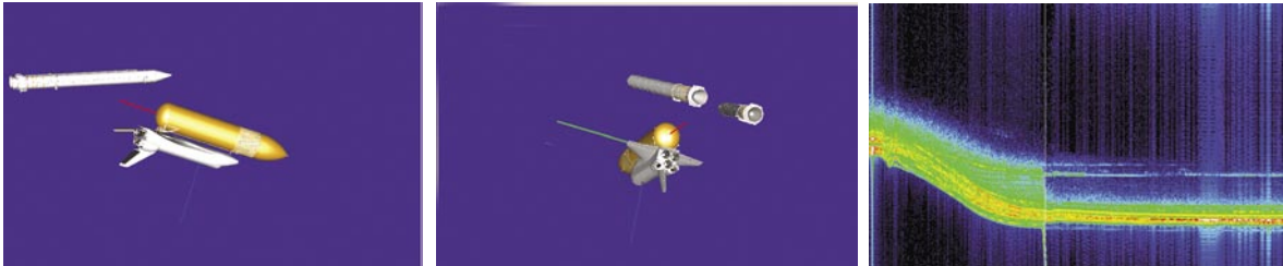
Pictured from left: The first and second photos show the solid rocket booster separation from the shuttle’s external tank from two different angles. The range-time-intensity plot with separation phase from NCAR radar is shown in the third photo.
