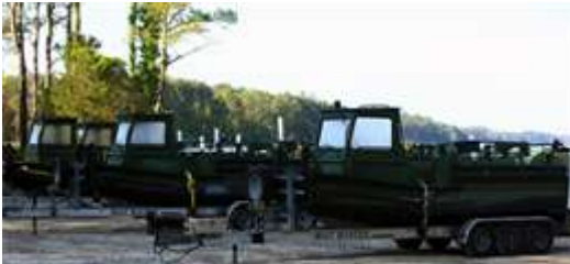
MK III Bridge Erection Boats belonging to 8th ESB, 2nd MLG sit at Engineer Point aboard Camp Lejeune, N.C., May 7, 2013. Approximately 15 soldiers with the Bermuda Regiment were instructed by Marines with 8th ESB to practice longitudinal and conventional rafting using MK III BEBs when building and using Improved Ribbon Bridges. (Photo by LCpl Devin Nichols)
