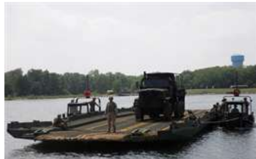
Marines with 6th ESB transport bridge equipment across a lake using an improved ribbon bridge during a training exercise here, June 11. The IRB uses a series of floating platforms to safely transport heavy equipment, supplies and troops across a large body of water. (Photo by Cpl John M. McCall)
