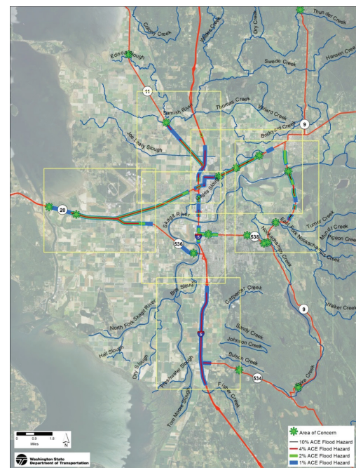
Figure 1. Map of the pilot study area with the flood hazard locations for the 1% (blue), 2% (green), 4% (red), and 10% (black) Corps’ annual chance of exceedance (ACE) floods. Areas of concern are denoted with a green asterisk.
