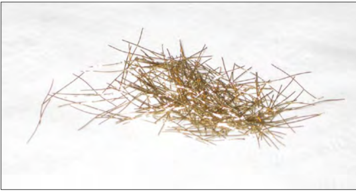
Steel fibers reinforce UHPC, which offers simple, durable connection details for prefabricated bridge elements.
