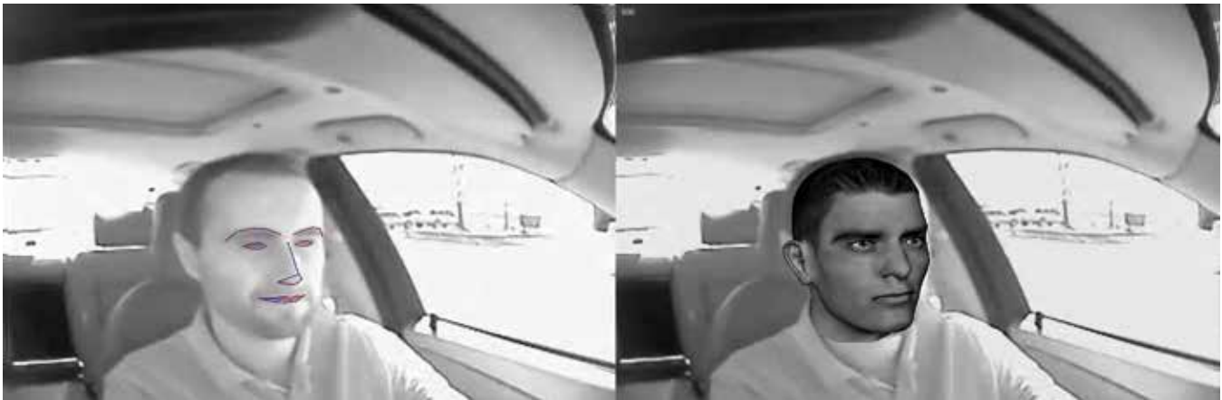
Figure 7. A driver’s identity is protected using an avatar to replace their face in all frames.
