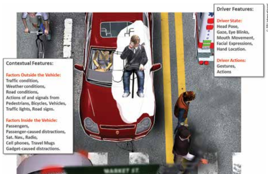
Figure 2. The DCode System will extract driver behavior features and recognize various actions. It will also track contextual features.
