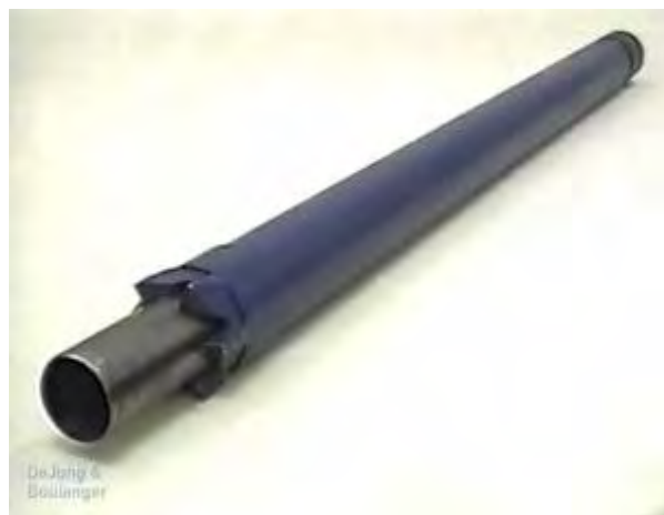
Figure 3-12. Pitcher sampler (FHWA, 1997, 2002b).
