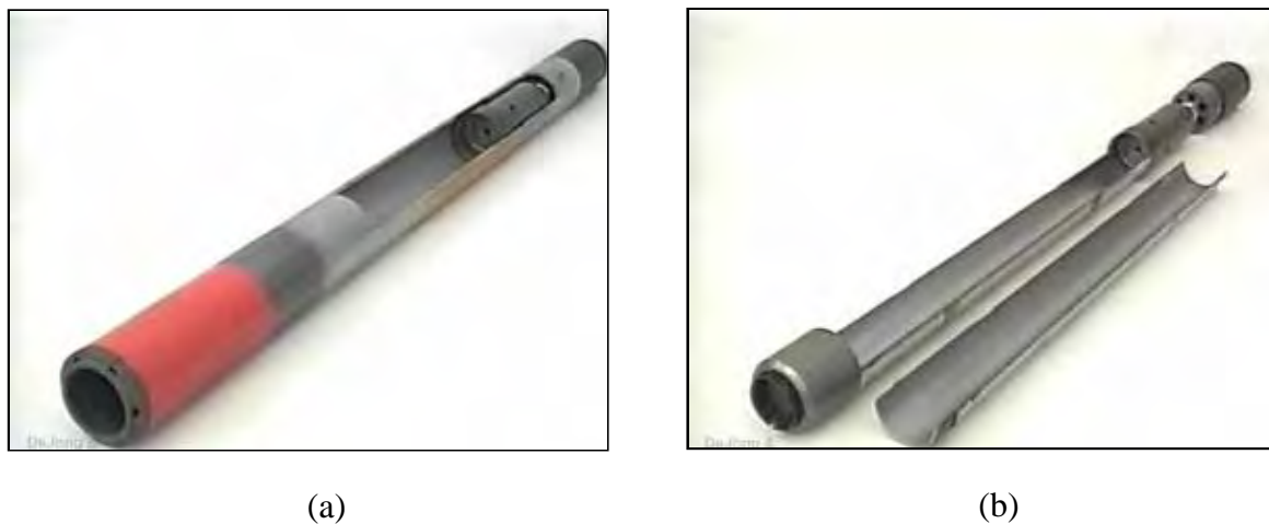
Figure 3-15. Double tube core barrel. (a) Outer barrel assembly (b) Inner barrel assembly (FHWA, 2002b).
