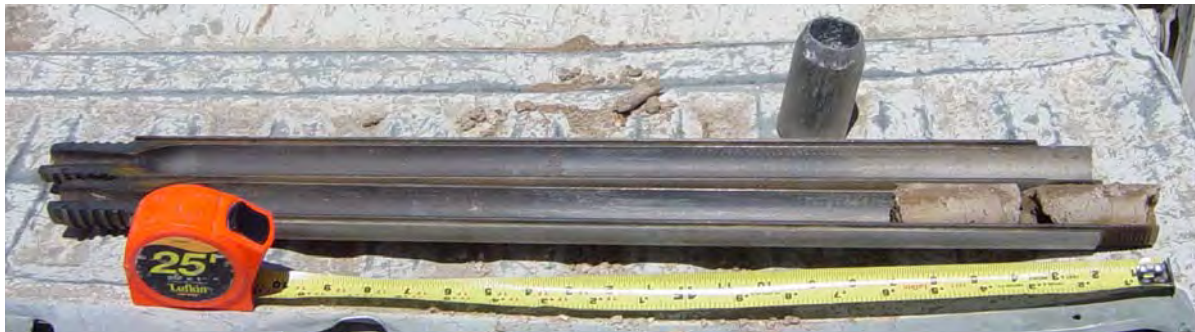
Figure 3-8. Split barrel sampler.
