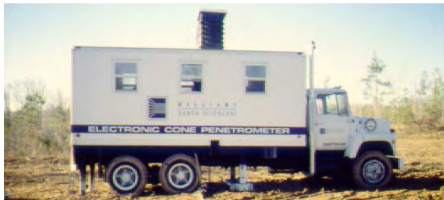
Figure 3-29. Cone penetration testing from cone truck.
