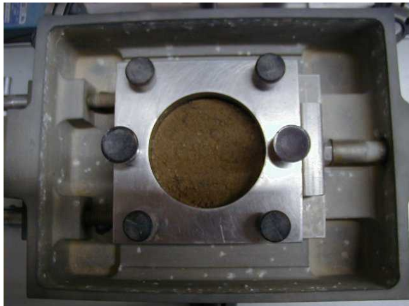
Figure 5-19. Soil sample mounted in direct shear testing apparatus (Photograph courtesy of GeoComp Corporation).
