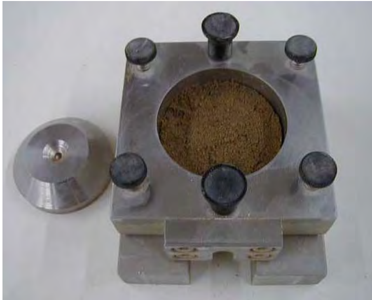
Figure 5-18. Direct shear testing box (Photograph courtesy of GeoComp Corporation).
