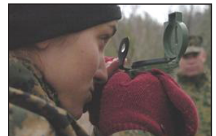
Marine shows the proper technique in shooting an azimuth using a lensatic compass.
